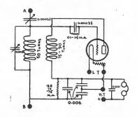
nal a means, well within the capabilities of most amateurs, whereby the results obtained by Armstrong can be approached, if not duplicated. The circuit reproduced has all the characteristics of the Super-regenerative circuit of Armstrong when in operation, such as the whistle, which has to be tuned out, and the tight coupling of the regenerator coil.
