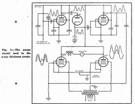
the two plates, any unbalance in the circuit will be indicated by a deflection proportional to the amount of unbalance. This unbalance, of course, will be caused by differences in amplitude of pulse "A" and pulse "B".
