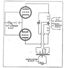
Fig. 6.—Basic arrangement of balanced modulator.
