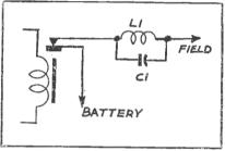
Details of the regulator filter. The coil, L1 consists of 25 turns, 22 SWG enam. wire, % inch dia., 34 inch long. The condenser C1, is a standard 455 kc. padder.
