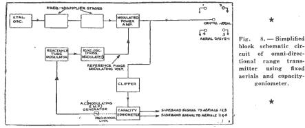
A straightforward method of approaching the problem would appear to be to set up a *figure-eight* aerial of one of the types just described, to apply a C.W. carrier to it, and to rotate it about a vertical axis by means of a motor at a speed corresponding to the modulation frequency it is desired to produce at the receiver. At the same time, the C.W. carrier would be fed to an omni-directional aerial which is stationary and mounted co-axially with the rotating aerial.
