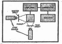
Fig. 2.-Block diagram of a one source-two pickup system.
