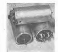
I.F.'s and Ratio Detector Coil
