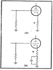
Fig. 2.—Negative feedback voltage may be developed across the cathode resistor of an amplifier by omitting the bypass condenser as shown in (A) or by placing the bypass condenser across only part of the cathode resistor as shown in (B).
