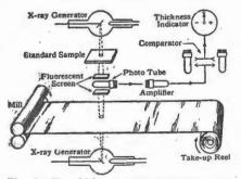
Fig. 1.—The thickness gauge uses two x-ray generators. The radiations from one pass through the sheet in question; those from the other through a standard. The surviving radiations fall, alternatively, on to the xradiation sensitive screen surrounding a photomultiplier. The results are amplified, compared, and any difference applied to an indicator. tube, and any variations in thickness of the sheet under test will be indicated on a suitable meter. The basic arrangement is shown in Fig. 1.
