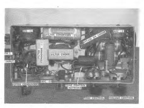
This underchassis photograph shows how most components were fitted in. This layout keeps all leads to o minimum, thus reducing one potential source of interference.
