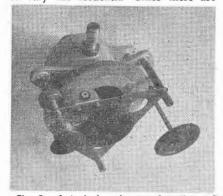
Fig. 9.—A typical cavity tuned oscillator for 1200 Mc/s operation using a GL-446B lighthouse triode.
