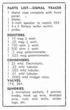
coupling condenser and 10 meg grid resistance, all mounted in the probe shield. The condenser acts as a blocking condenser isolating any DC voltages from the input circuit, whilst the 10 meg resistor acts as a grid return and bias resistor. This high value also means that the input impedance of the grid circuit is kept high, thus reducing any loading effect on the circuit under test to a low value.
