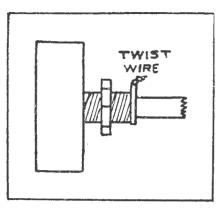
Twisting a piece of wire around the volume control shaft will often cure  $\alpha$  "noisy" control.
