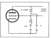
Fig. 11.—The Barkhausen and Kurz positive grid oscillator circuit.
