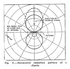
A reflector is simply another rod which is placed parallel to and in back of the receiving dipole. The reflector element is usually about 5 per cent. longer than the receiving dipole and is placed about  $\frac{1}{4}$  wavelength in back of the receiving dipole with a resulting gain in signal pickup of about 3 db in the direction in which the broadside of the receiving dipole is pointed; a half-wave dipole with a reflector is shown in Fig. 6.
