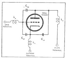
Fig. 1.—Equivalent circuit of a triode at U.H.F.
