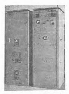
Radar beacon at Georges Heights, Sydney. The transmitter is on the left, the receiver and associated units on the right.
