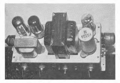
A top view showing the chassis layout. The vibrator and rectifier are mounted on the right, and the amplifier section at the left.
