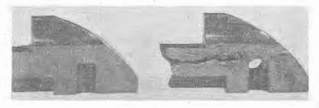
This photograph of bakelite moulding samples with and without H.F. preheat, clearly illustrates the effectiveness of this method of heating.
