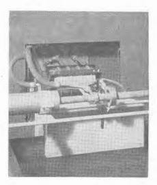
Experimental arrangements for deep surface hardening of gudgeon pins using 70 kw. H.F. Induction Heater, showing coupling transformers for obtaining high work coil current.
