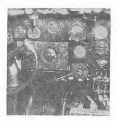
Instrument panel of Skymaster aircraft; distance indicator can be seen immediately in front of the throttle column.
