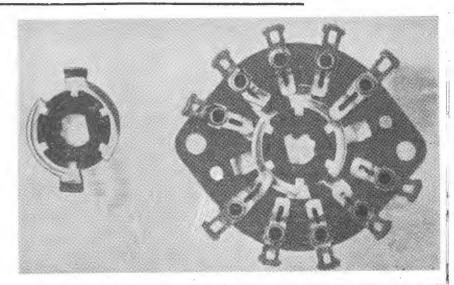
Photograph of a typical wafer switch, subjected to mechanical life test after cleaning with carbon tetrachloride.
