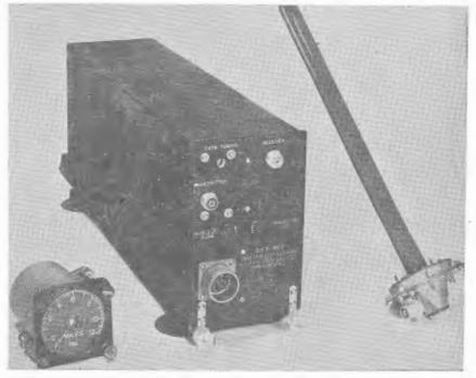
Engineered prototype model of the Australian Distance Meosuring Equipment, showing the main unit, a distance indicator and aerial.
