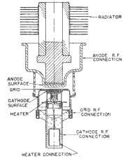
Fig. 3.-A sectional drawing of the 2C39.
