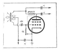
The audio oscillator circuit. Any triode or pentode connected as a triode will operate satisfactorily.
