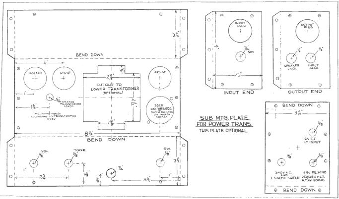
The necessary chassis dimensions are given in this drawing. Note the optional mounting for the power transformer.
