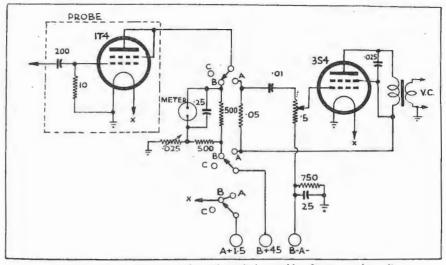
Although only requiring two valves, the unit is capable of very good results.
