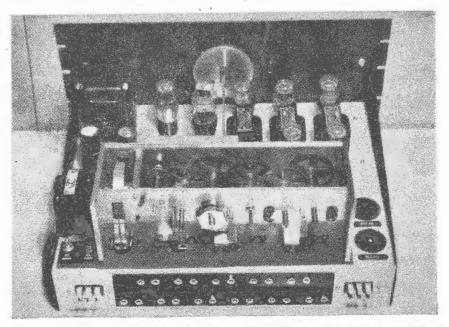
The Seconds Pulse Generator and time interval selector used in the time control equipment at station WWV. The one second contact is made by a cam on the flywheel immediately at the right of the electric motor.
