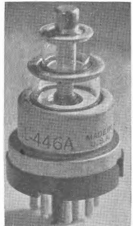
The unique construction of a "lighthouse" tube is clearly shown in this excellent photograph.
