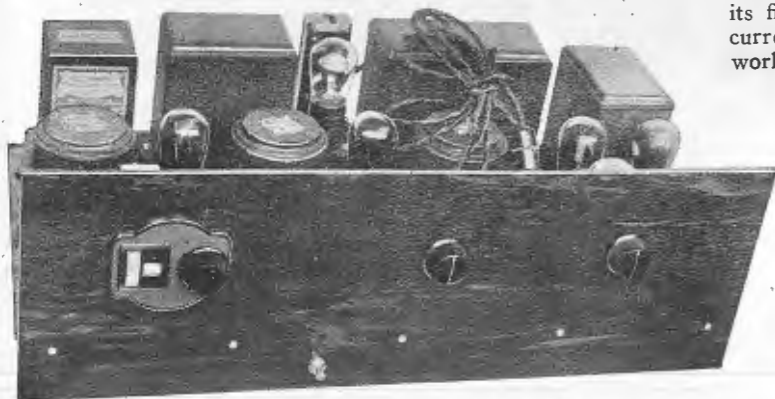
FIG. 1.—Front elevation of the 1929 Electric Solodyne. On the front panel is mounted, from left to right, the single tuning dial with drum indicator; the power switch; the reaction control; and the volume control. The baseboard is attached to the panel by means of the five screws shown. Over the panel may be seen the tops of the three shielded coils, five valves, the power pack and the output filter.
