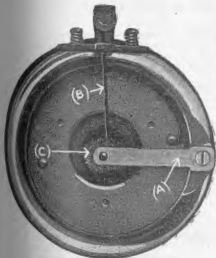
This photograph shows the damping spring (A) and stylus bar (B) in position. The small felt pad (C) is secured to the end of the damping spring, applying pressure to the point where the stylus bar and driving unit are joined. The spring may be secured to the unit either by means of a small machine screw or solder.
