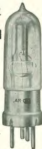
TYPE "A. R. 06." Filament Voltage, 2.5. Plate Voltage, 20-50. Filament Current, .06 amperes. Price, 1s/6 each.
