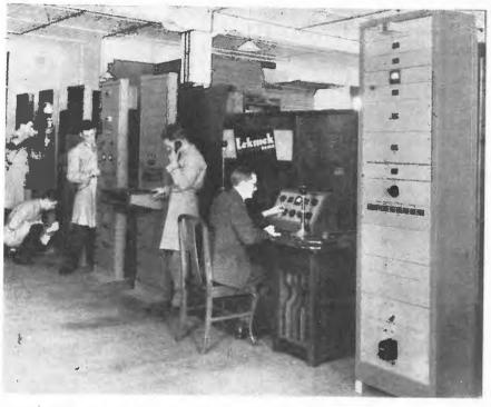
Almost ready for shipment. Some of the racks for new "A" Class Station on the left of photograph, and complete Amplifier Cabinet and Announcer's Control and Desk for new Mudgee Commercial Station on the right.
