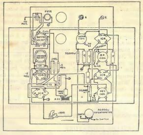
Base lay-out plan and picture diagram of the wiring for the "Sky-Cruiser" battery set.
