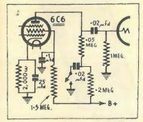
tor used for the 6C6 in the original circuit of the "Fidelity" is replaced by two resistors in series, with values of .05 and .2 megohm. From the junction of the two a condenser of .02 mfd. is taken to earth through a switch. With the switch open, all frequencies are amplified uniformly, but with it closed the higher audio frequencies are by-
