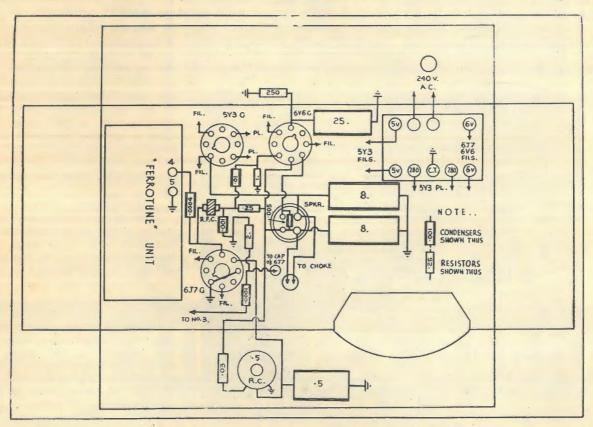
Compare this diagram with the photo opposite and the wiring is easy.
