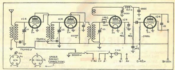
The "Sky-Cruiser" circuit, showing all values. Three 1C4's and a 1D4 are used.
