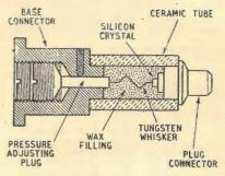
its early prototypes. As the sectional drawing in Fig. 1 shows the crystal and tungsten catswhisker are contained in a small ceramic tube closed at each end by brass plugs and completely filled with wax. This form of construction results in a mechanically robust device in which the contact is quite undisturbed by normal shocks.
