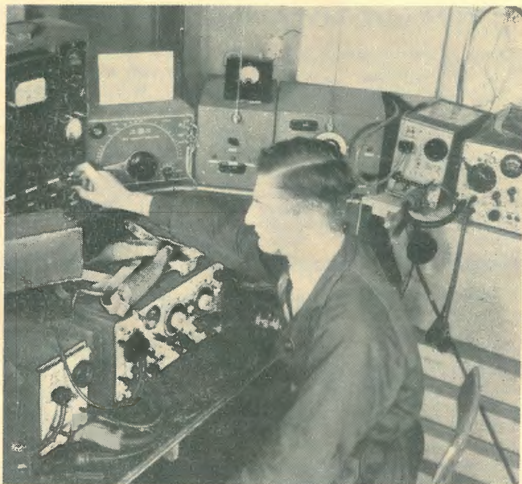
Only yesterday! This "shot" was taken during the war at an Australian Army Inspection test room at a large radio factory. It shows final checking in progress on "Wireless Set 22," a conspicuously successful field radio equipment as used by the A.I.F.
