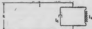
Fig. 1. Circuit of inductor and capacitor in parallel. At resonance I_k = -I_c , and I = 0 , since there is no resistance in the circuit
