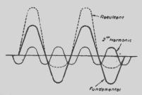
fundamental with its second harmonic produces the broken curve. Fig. 2 -- Combining o
