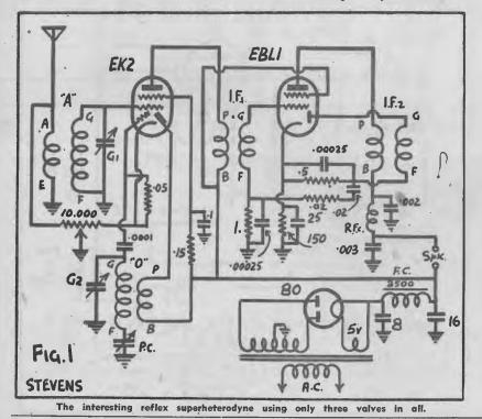
connect the oscillator plate directly on ot it, thus saving another resistor and condenser. The power of this set is equal to any good 4-valve of stan-dard design due to the high conductance of the EBLI, the current consumption low enough for a 40 Ma. power transformer.
