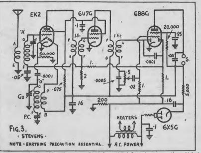
A suggested circuit, taking the power direct from the A.C. mains, a practice which is NOT recommended unless special earthing precautions are taken to avoid danger.
