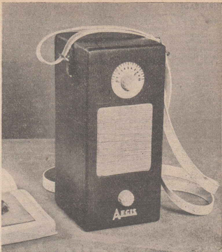
The Aegis Personal Portable receiver which is detailed in this issue. The kit is available as a four-valve model, with an auxiliary kit to convert to a five-valve circuit at a small extra charge.
