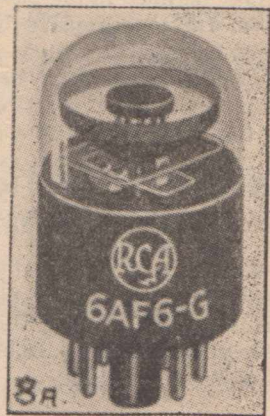
The compact size of a typical dual tuning indicator compared to the earlier shaded sector types is clearly illustrated in this photograph.
