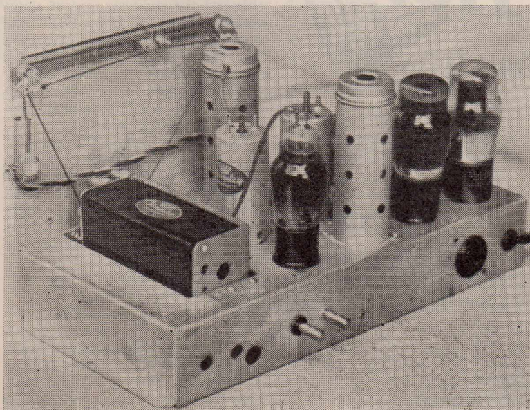
Rear view showing the "Ferrotune" unit fitting through the chassis.
