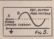
pulses or transients are received, the detector rectifies them, and reproduces their wave form as large negative voltages. These voltages reduce the limiter plate current to zero and the result is that no noise larger than the signal can pass through the limiter and be applied to the A.F. amplifier.
