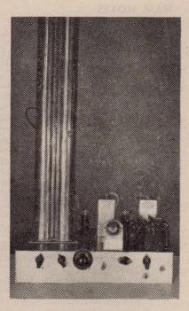
This example is of a modern coaxial-tuned V.H.F. Receiver. High frequency is obtained in the input circuit by the use of the concentric line.
