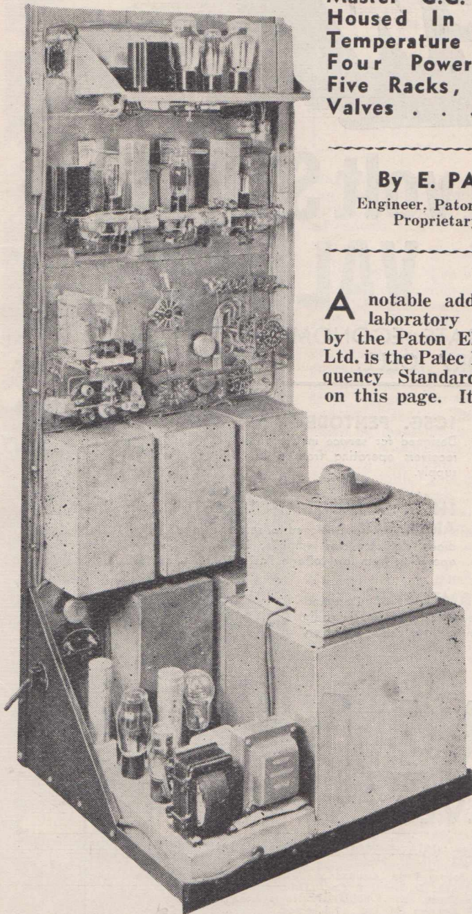
The photograph above shows a general view of the instrument, while on the left is a rear view, taken with shield covers removed. The box on which the large dial is mounted horizontally is the constant temperature oven.
