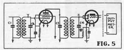
steps to prevent D.C. operating the meter, and measure a constant input signal as found at these two points. If required, various frequencies may be used and a "response curve" of the stage or stages obtained.
