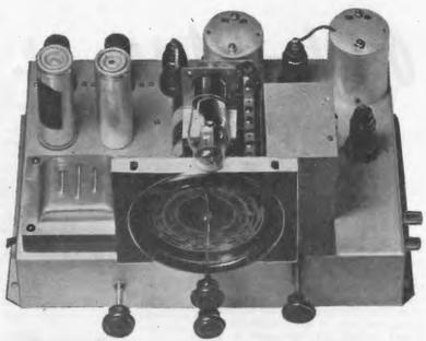
ference was high, all the main inter-State stations could be received quite comfortably after three o'clock in the afternoon. London and Paris were also received at full volume, but were badly interfered with by local elec-trical noises. Even under these conditions, however, the "Air Commodore" showed a better signal-to-noise ratio than three other A.C. ceivers (two five-valve superhets and one six-valve) tested at the same time.
