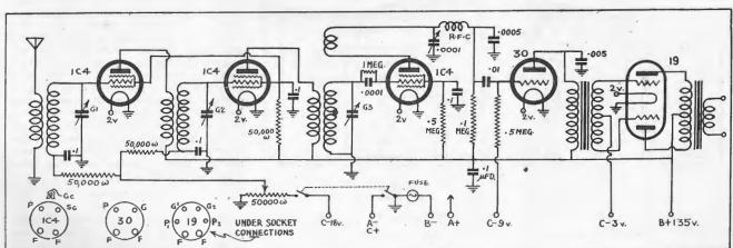
The amended circuit differs from the original only from the grid of the stage following the detector, onwards.
