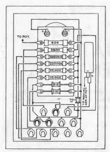
Fig 3.—This sketch shows the complete wiring, which can also be seen in the sub-panel photograph.
