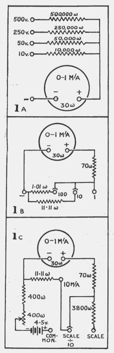
R1 = 1000 E, where R1 is the series resistor and E, the maximum voltage to be measured in each case. Thus, for ranges of 0-10, 0-50, 0-250, and 0-500 volts, series resistors of 10,000, 50,000, 250,000, and 500,000 ohms are required. A sensitivity of 1,000 ohms per volt is obtained on all voltage readings.
