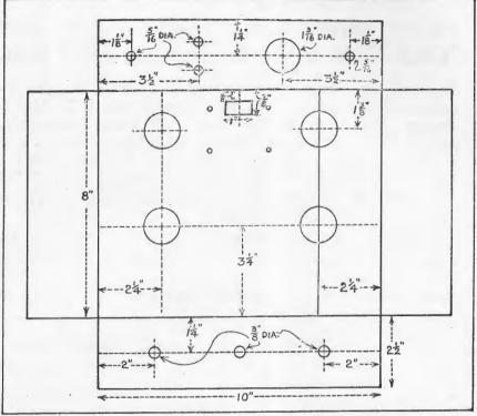
Dimensions for stamping and drilling the chassis, which is of 18-gauge steel, are shown above.
