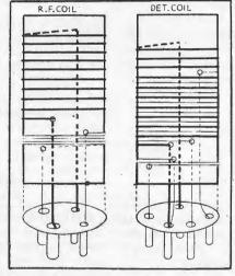
The method of winding the coils, and the connections, are shown in this sketch.
