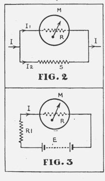
is given in ohms per volt; in this case, it is  $\frac{1}{.001}$ , or 1000 ohms per volt.
