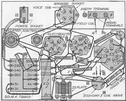
NOTE: THE FILAMENT WIRING TO THE 2AS E.53 VALVES HAS BEEN OMITTED HERE. CONNECT UP THE 2150 4A LUGS ON TRANS-FORMER TO THE "F" LUGS ON THE TWO VALVES; TWIST THE WIRES TOGETHER
