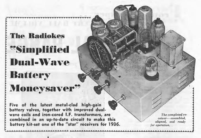
A YEAR or so ago it was impossible to design a battery receiver that would give results comparable with those obtained from an a.c. operated set using an equivalent number of valves. To-day, however, with the introduction of new high-gain 2-volt valves, this is no longer true.
