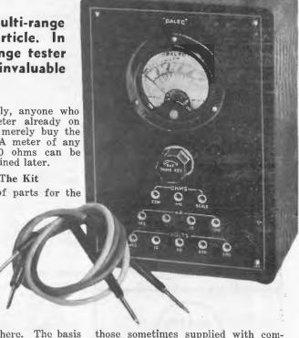
tester is shown elsewhere. The basis of the instrument is a Palec 0-1 milliammeter - a precision-built, highgrade meter that can be depended on to give high accuracy and trouble-free service.
