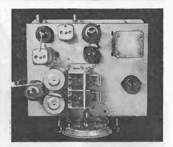
Right: This plan view shows the well-spaced layout. The special iron-cored I.F.'s are housed in attractive square cans.
