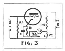
Last month the principle upon which the vacuum tube voltmeter operates was explained, and the features necessary in an instrument designed for service work outlined. In the concluding instalment below, a few of the varied uses of a V.T. voltmeter are indicated.
