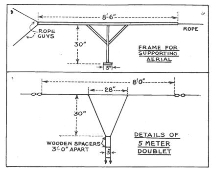
Details are shown above of the aerial and aerial support, which are mounted vertically
