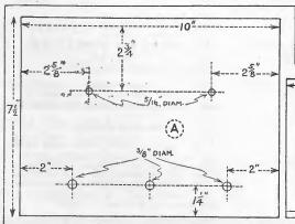
Sketch A (left) shows dimensions for preparing the front panel, B and C, for the aluminium shield partitions, while D gives details of the bracket for mounting the r.f. valve under the chassis. All flanges shown should be \(\frac{2}{3}\)in. wide. The chassis layout is shown elsewhere.
