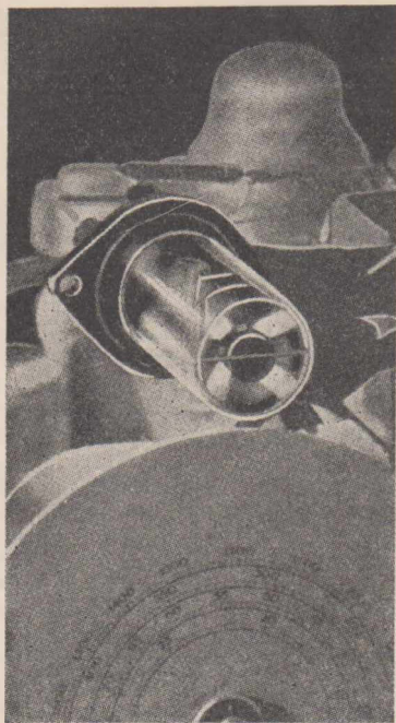
This photograph shows the EM1 incorporated as a tuning indicator in an ordinary receiver chassis.
