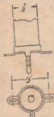
Type 51-134. Flanged Clamp—used where above chassis mounting is required and capacitor is earthed. Capacitor body is not insulated.
