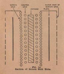
For radio-frequency purposes it is necessary that the grid-plate capacity be small to prevent feedback and self-oscillation, otherwise full use could not be made of the high gain of the tube. The gridplate capacity of this type of tube is small, due to the reduction of the space charge.
