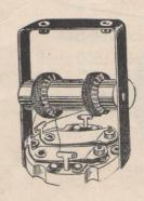
Same design as 5-10, but is 465 KC, and uses Isolantite two-plate tuning base, type B2 (see I.F. tuning condensers). It is a very efficient high gain I.F. transformer, suitable for single stage amplification, following 2A7 or 6A7 valves. Is also very efficient when used with 57 or 6C6 autodyne oscillators, provided the oscillator coil is correctly designed and the correct values of cathode resistor and bypass are used.
