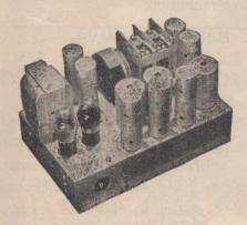
We recommend this kit to anyone wanting a radio set to cover all wave lengths from 15 to 550 metres. In all Radiokes all wave sets the coil assembly is wired, completed, tested and sealed, making it a very simple matter for the constructor to assemble the Kit-Set. There are no complicated switches to wire—we do all that for you.
