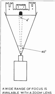
Each lens subtends or accepts a certain angle of vision which can be measured in degrees. This is true for all lenses whether fitted to film, ENG or studio cameras. For example a wide angle lens may encompass a horizontal angle of 400, the outer edges of its angle of vision radiate forwards and
