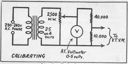
Set-up for calibrating the meter.
