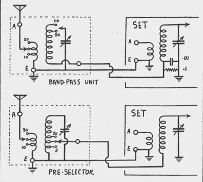
coil and condenser should be of the same types as in the receiver. If these cannot be obtained then a coil can be wound as shown in the diagram, and a good-quality secondhand variable condenser of about .0004 to .0005 mfd. maximum capacity will do the trick.
