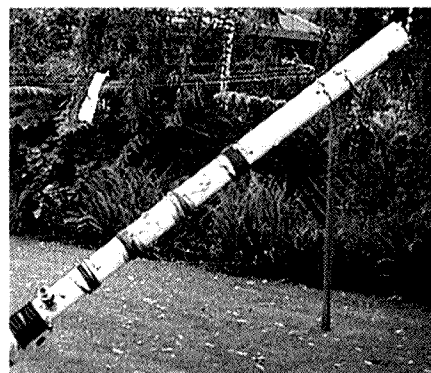
Photo 1 - The 10 m EH antenna.
