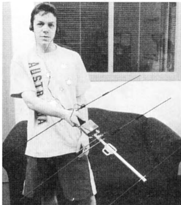
One of the WIA junior team Nathan Wyss checks out an ARDF sniffer ready for action.
