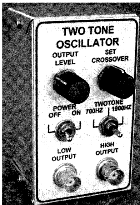
Photo 1 - The Single and Two Tone Generator.
