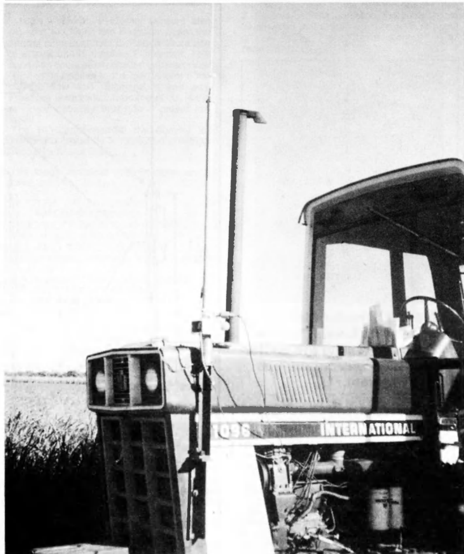
The Base of the Antenna. Note the SO239 to connect the coaxial cable.
