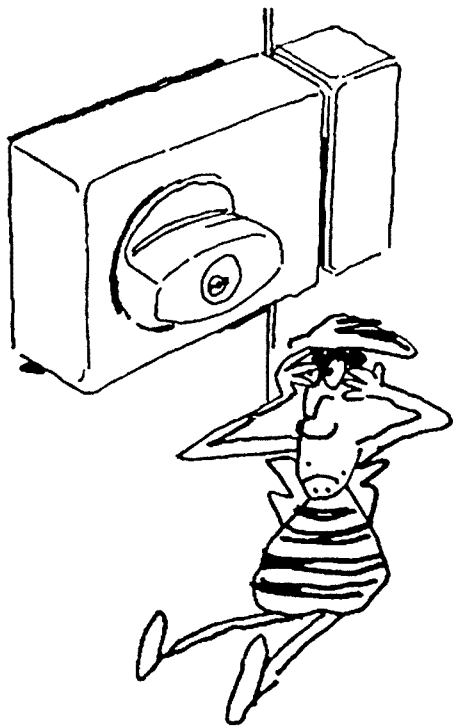
This is a double cylinder automatic deadlatch (screwed to the inside of the door) and is a cost effective fortification.
