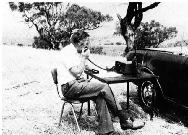
Bruce VK3UV with helical whip and FT101 amongst the big signals on 14 MHz.
