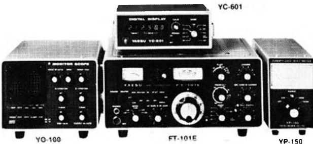
As shown in the photograph is the YO-100 monitor scope, FT-101E transceiver, YC-601 digital readout adapter and YP-150 dummy load-power meter.
