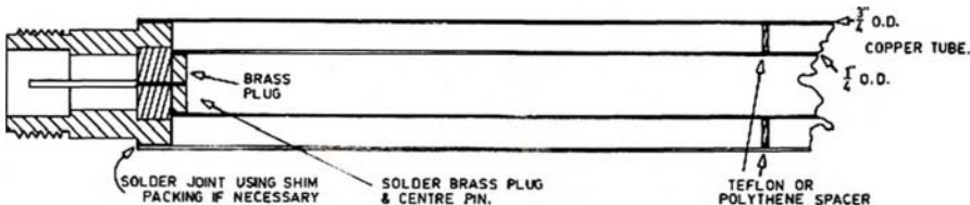
Fig. 2.—Assembly of Type N Connector to Copper Co-ax.
