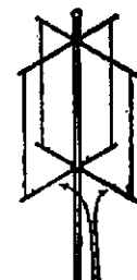
Fig. 12—Tapping points along the radiators permits selection of impedance from 50 to 600 ohms.
