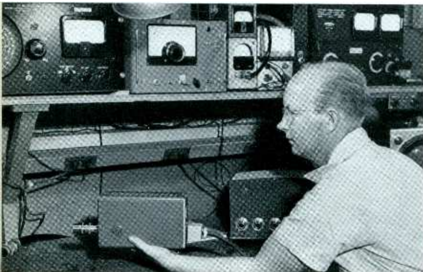
This RCA "TV Eye" camera is the heart of a closed-circuit television system used in business and industry.
