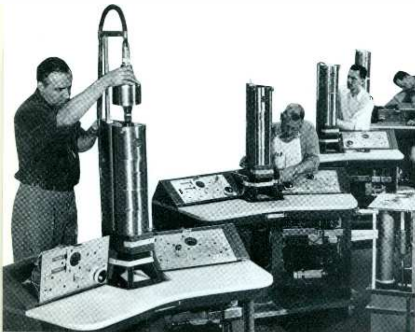
RCA electron microscopes nearing completion at Camden, N. J., plant of Engineering Products Division. The instruments are used extensively for research in the fields of chemistry, metallurgy, medicine, bacteriology and biology.
