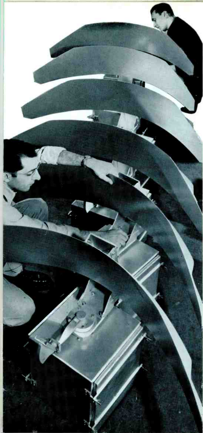
Making final adjustments on radar antenna units for small craft vessels at Radiomarine plant in New York City.
