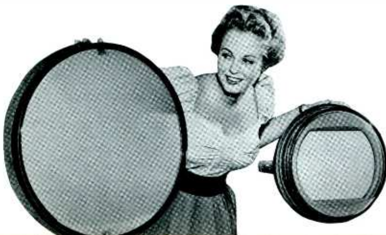
New RCA 21-inch color TV tube is shown in comparison with the earlier 15-inch color tube.
