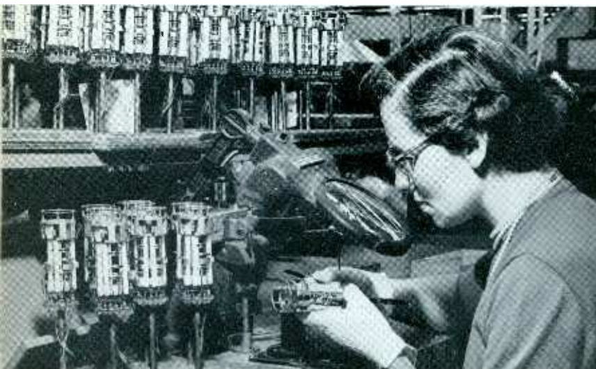
Delicate parts used in electron gun of a color television picture tube are assembled under magnifying glass.
