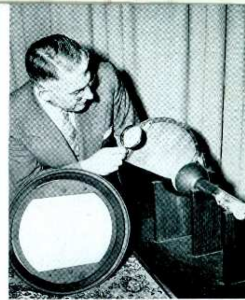
Cut-away view of RCA's tri-color television picture tube shows the screen with its 600,000 dots of phosphors.
