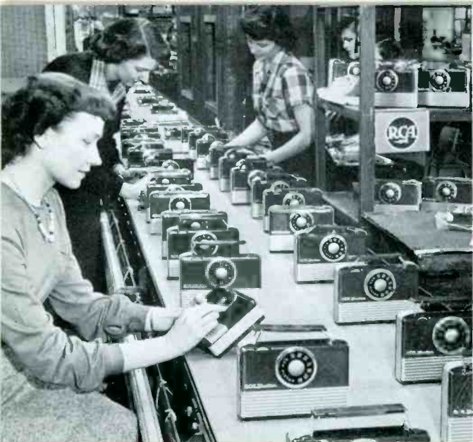
RCA's book-size personal radio sets undergo final inspection as they move down production line at Canonsburg, Pa.
