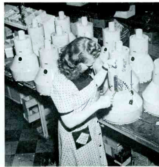
Attaching terminal blocks to the metal shields of 12-inch scopes of Radiomarine's large radar units.
