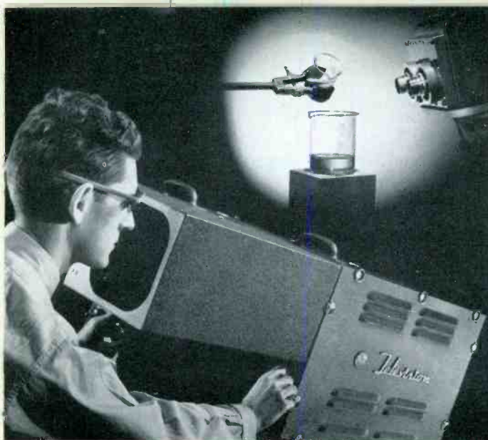
RCA's industrial television system can be adapted to provide a stereoscopic view of a remote-controlled chemical process.
