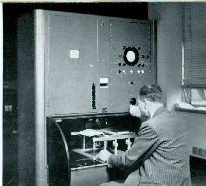
High-speed facsimile system developed by RCA for the distribution of printed matter at the Oak Ridge National Laboratory.
