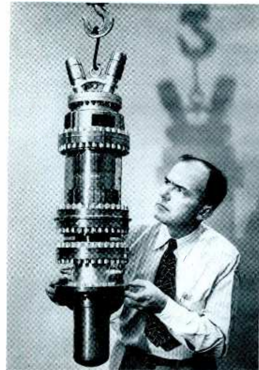
RCA's "Super-Power Beam Triode" is capable of delivering 500 kilowatts of radio-frequency power.
