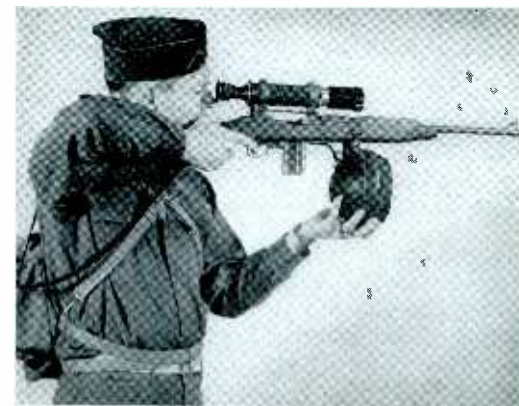
Infra-red image tube, developed by RCA, is the heart of this sniper-scope which permits riflemen to see targets in total darkness.
