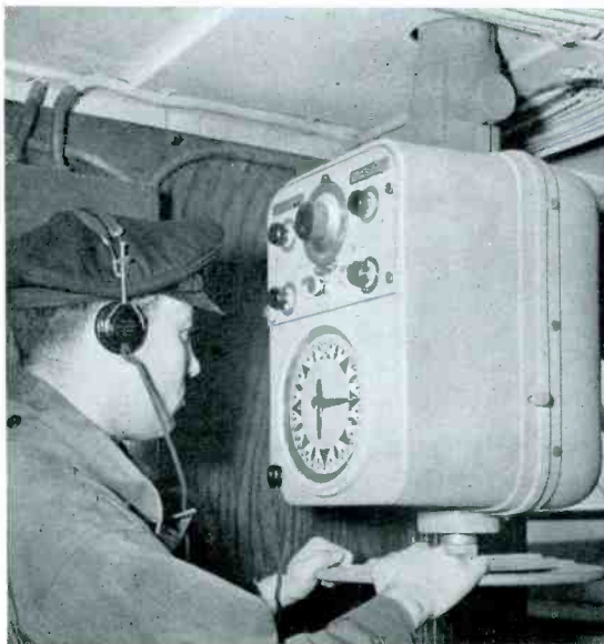
Radio direction finder, designed and built by Radiomarine, is installed in the chart room of an ocean freighter.
