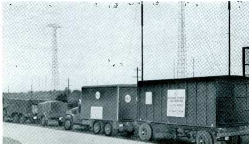
Four units of a mobile radio station sent to the Korean fighting front by RCA Communications.
