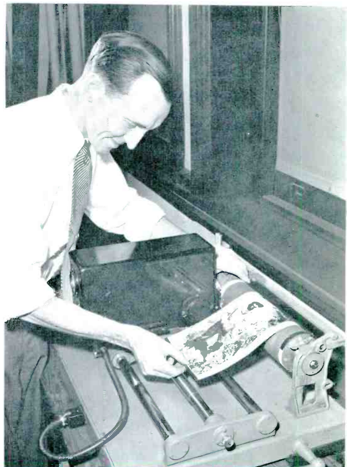
Photographs, drawings, and documents travel thousands of miles in a few minutes over RCAC international radiophoto circuits.
