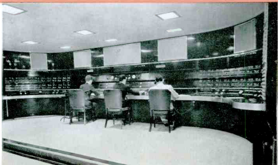
The master control board of NBC is a central point where stations scattered across the country are linked with Radio City to form a nationwide network.
