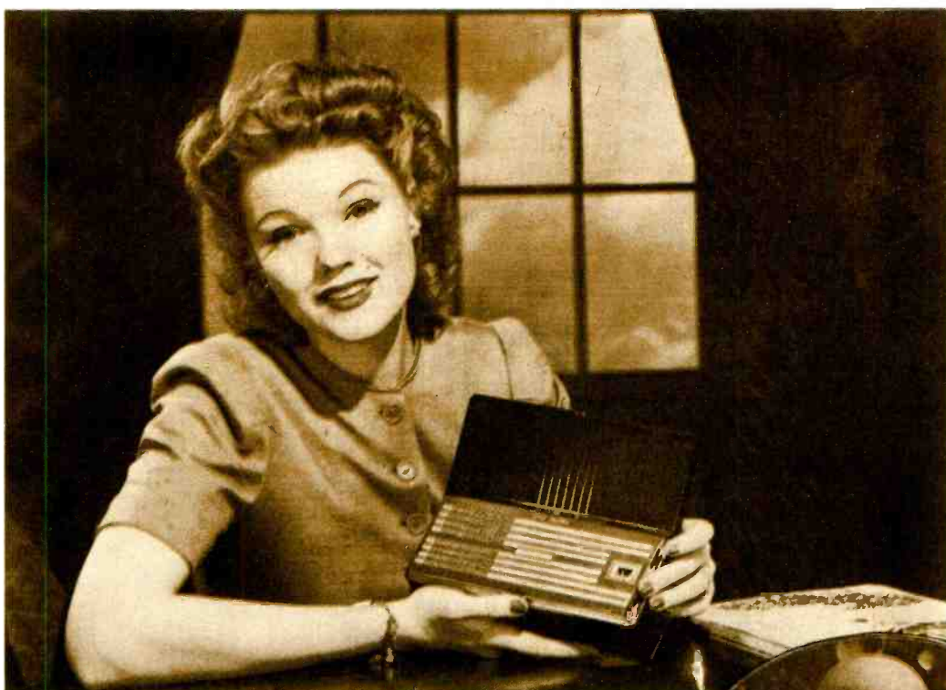
The RCA "personal" radio, made possible by the development of tiny tubes and miniature components, appeared prior to the war, and was a forerunner of wartime portable equipment.
