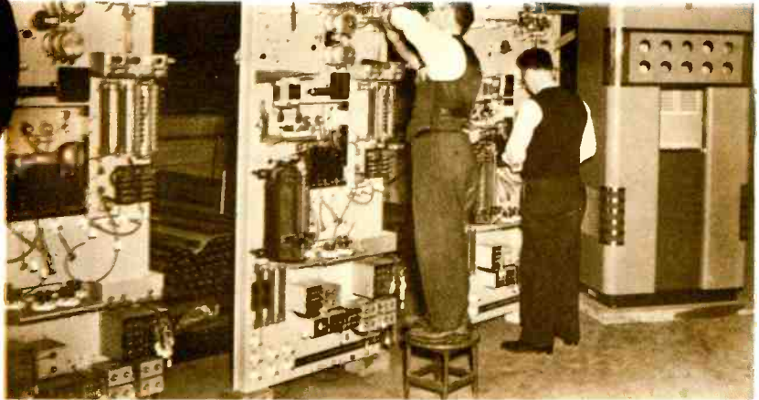
Radio apparatus of all types is produced by RCA; here 250-watt transmitters are being assembled.
