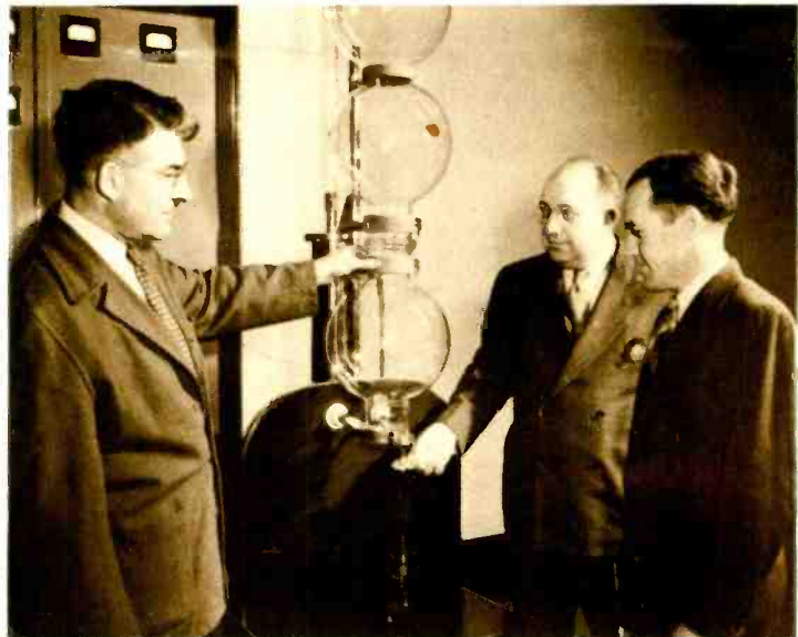
BELOW: Cyril N. Hoyler, Dr. George H. Brown, and R. A. Bierwirth, of RCA Laboratories, with the electronic dehydrator which they developed to speed production of penicillin.
