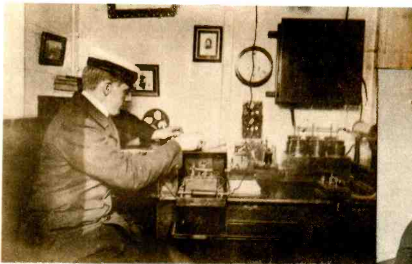
ABOVE: Early shipboard radio apparatus, as installed on the SS Minnehaha in 1904, featured a coherer with tape recorder and a spark-coil transmitter — a marked contrast with the modern, compact marine apparatus which utilizes electron tubes and establishes communication with land from any latitude-longitude on the Seven Seas.
