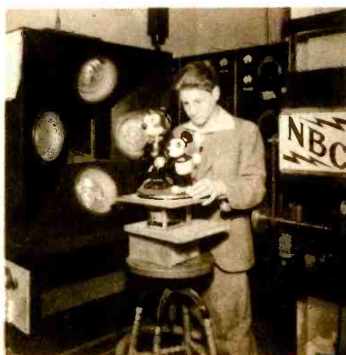
ABOVE: In the late Twenties, Felix the Cat and Mickey Mouse whirled for hours on a phonograph turntable in front of television "eyes," while engineers in the field made reception tests.
