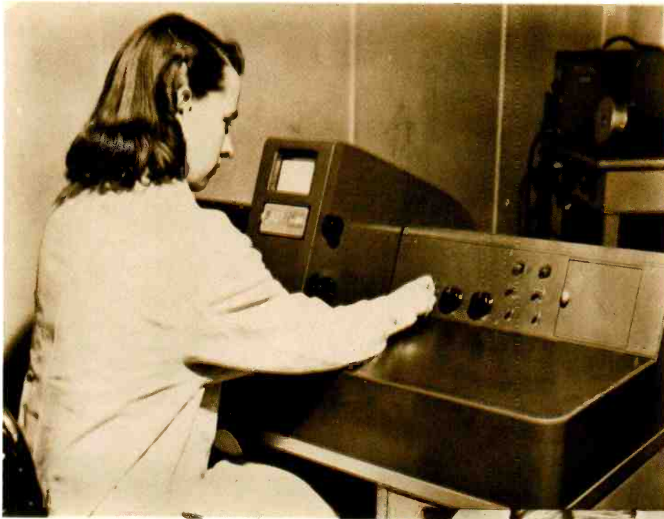
Console model of the RCA electron microscope enables photographic enlargement up to 100,000 diameters, depending on the subject matter. RIGHT: The windpipe of a mosquito magnified 65,000 times.
