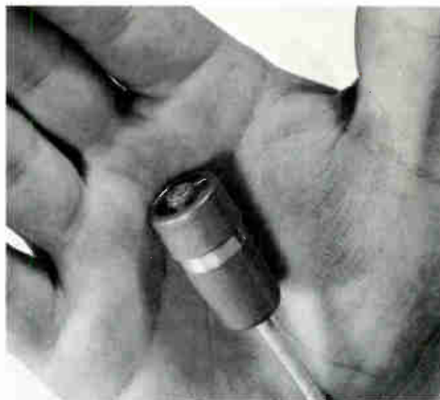
RCA's BK-12A subminiature lavalier dynamic microphone weighs less than \frac{3}{4} ounce and measures only 1\frac{1}{2} inches in length and \frac{3}{4} inch in diameter. Frequency response of this instrument covers the range from 60 to 18,000 cps. Special voice coil permits use with 30-to-250-ohm inputs without changing the microphone's impedance.
