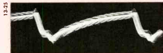
8E. The horizontal sync pulses move through the pattern, as indicated here, when the horizontal oscillator is out of sync.
