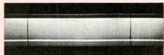
8H. Normal waveform, without a TV signal. (The two thin dark vertical lines in this and other photographs are made by two guide lines on the CRO screen.)
