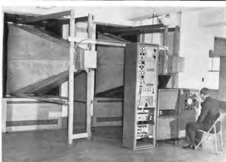
These devices that look like loudspeaker baffles are used to direct 506 Mc waves to a dipole antenna located in the small end. They are protruding from windows of the 62nd floor of the RCA building in New York and are receiving from Bellmore, Long Island.
