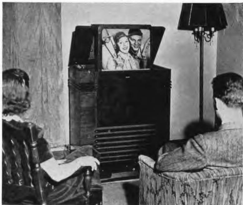
RCA has developed this home type television receiver which projects a picture on a screen 13½ x 18 inches.
