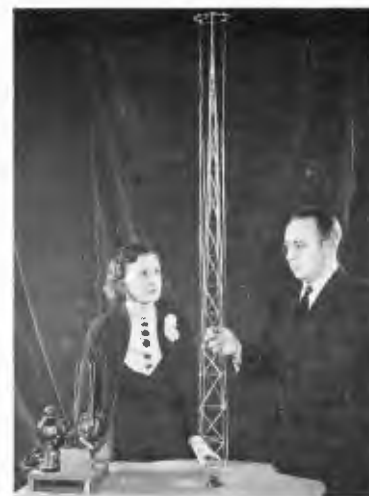
Dr. G. H. Brown, Research Engineer of the RCA Victor Laboratories, demonstrates an experimental model of a new transmitting antenna, designed to have a uniform electrical cross section.
