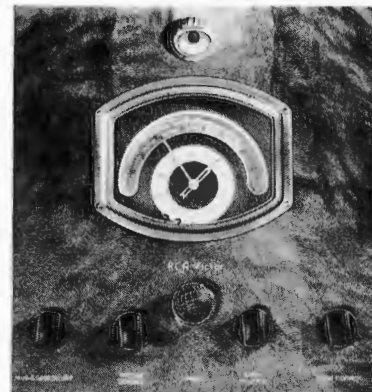
Above is shown the handsome control panel of one of the new RCA Victor receivers. Note the Magic Eye and the easily-read Selector Dial.
