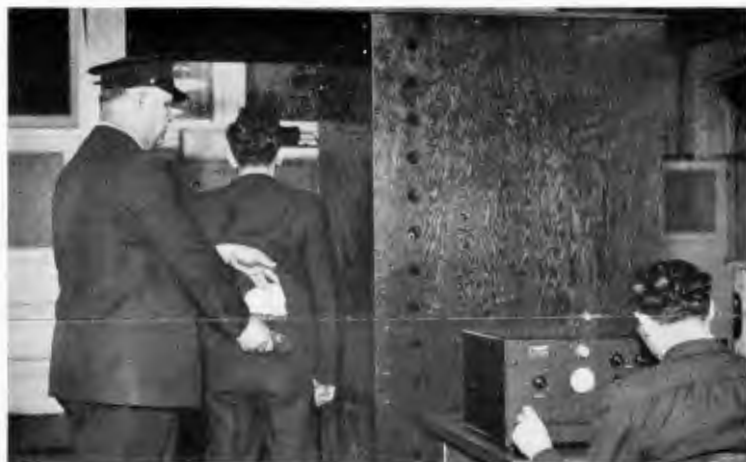
The new weapon detector foils jailbreakers by detecting any metal weapons accomplices might be carrying as they pass the device.
