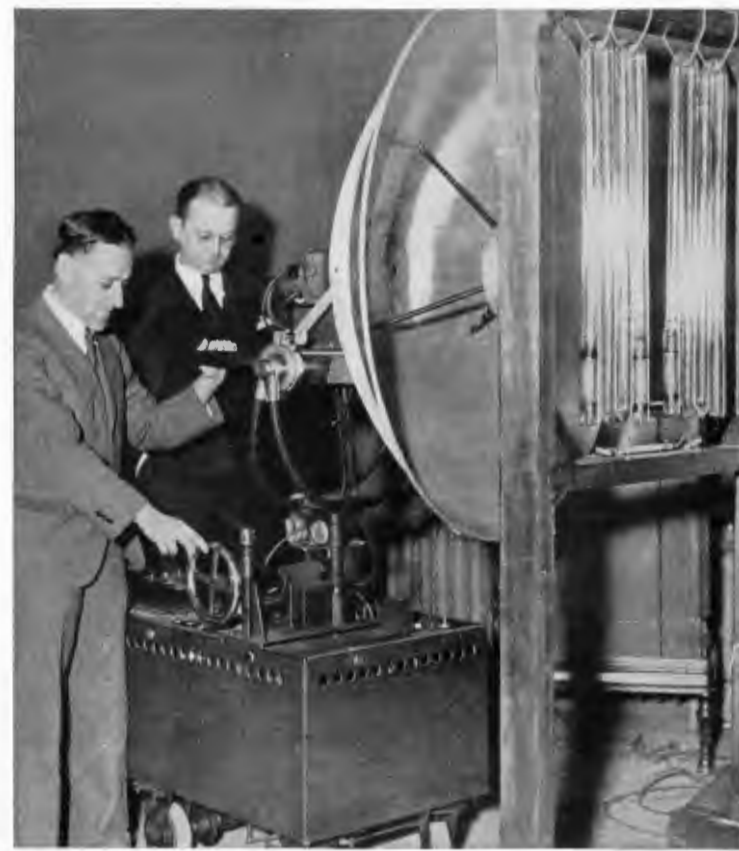
Dr. Irving Wolff, RCA Victor Research Laboratory, demonstrates a new ultra-short-wave directional transmitter of 9 cm., modulated by means of gas-filled tubes. The varying illumination of the tube corresponds to voice or music frequencies.
