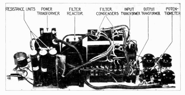
Figure 17-View of R.P.A. unit with cover removed
