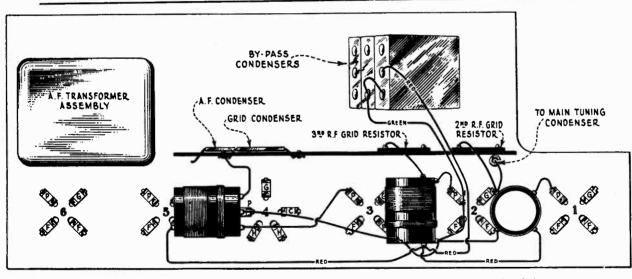
Figure 20-R. F. transformer connections and color scheme of wiring.
