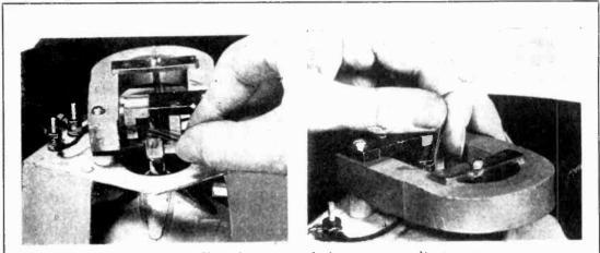
Figure 11-Use of spacer tools in armature adjustment
