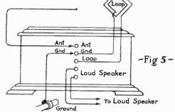
will usually serve the purpose. In making the ground connection, the pipe should be scraped clean and the ground wire firmly connected.
