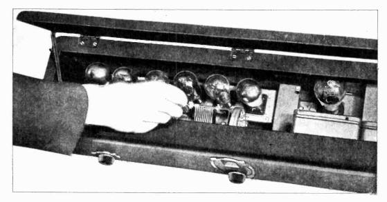
Figure 6-Adjusting the compensating condenser.
