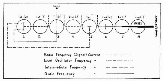
Figure 1-Radiola 28 Radiotron sequence
