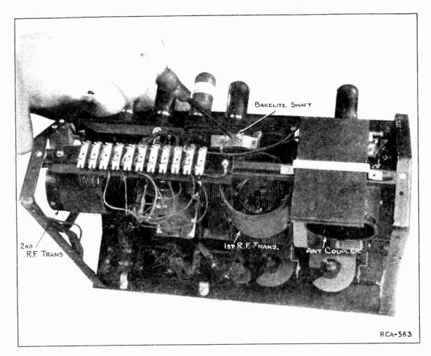
Figure 6 Adjusting the second neutralizing condenser
