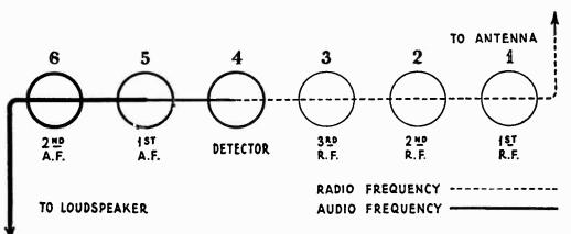
Figure 4—Radiotron sequence in RCA Radiola 18.
