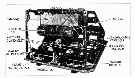
Figure 2-Rear view of panel assembly
