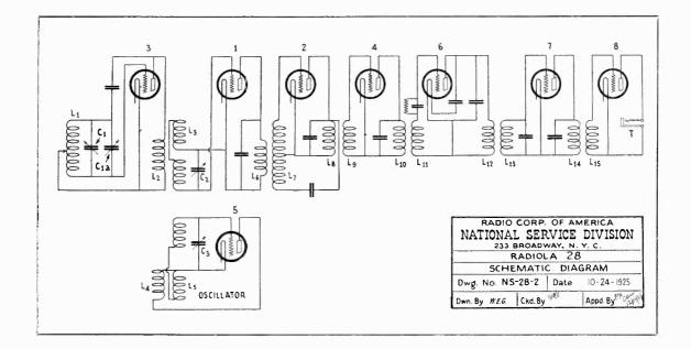
This circuit diagram is not intended for use in checking continuity tests. Use the continuity wiring diagram illustrated in Figure 7, page 12, for such tests.
