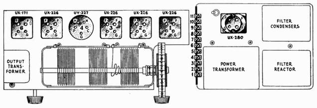
Figure 5—Radiotron socket contacts.
