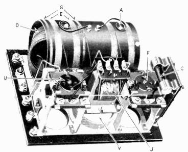
Fig. 7-Working Parts of Radiola RS
