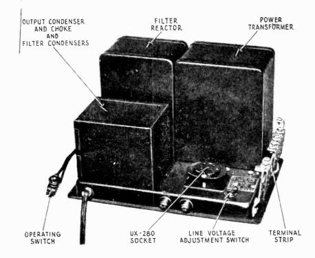
Figure 2-Socket power unit showing various parts.
