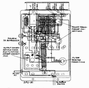
Fig. 8—Bottom of Socket Power Unit Showing Wiring Between Terminals
