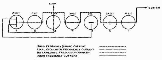
Figure 2-Radiotron sequence and path of the different currents
