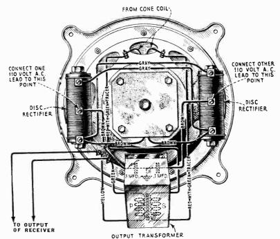
Figure 3-Wiring diagram of reproducer unit
