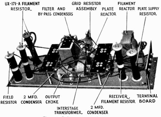
Figure 4-Socket power unit, showing parts
