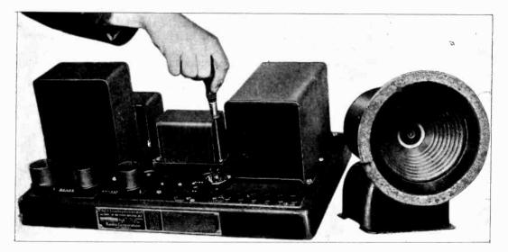
Figure 11—Removing output transformer.
