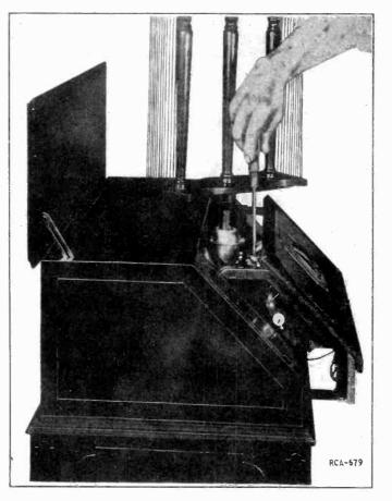
Figure 5—Adjusting the loop compensating condenser
