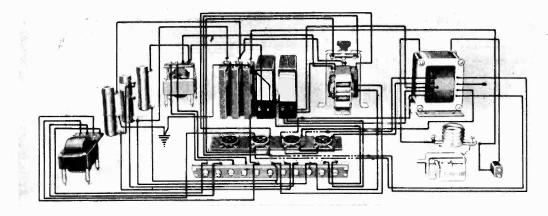
Parts and Wiring of Power-Amplifier Units
