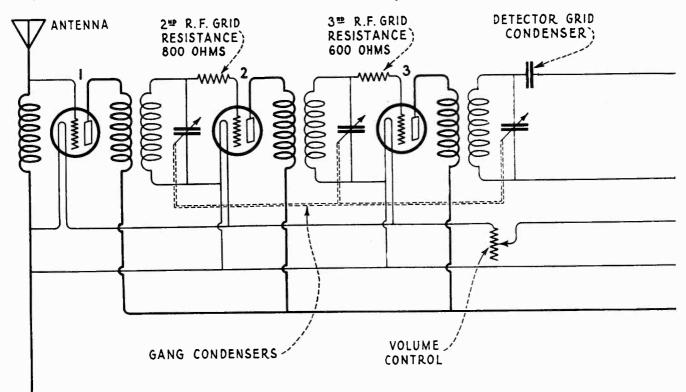
GROUND TO FRAME Figure 5-Schematic circuit diagram of RCA Radiola 16
