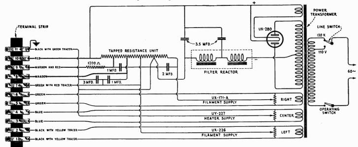
Figure 4A—Schematic circuit diagram of socket power unit.
