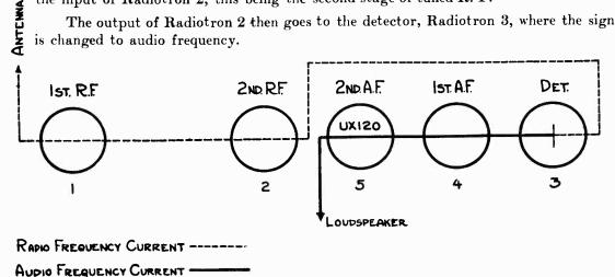
Figure 2-Radiotron sequence in RCA Radiola 20
