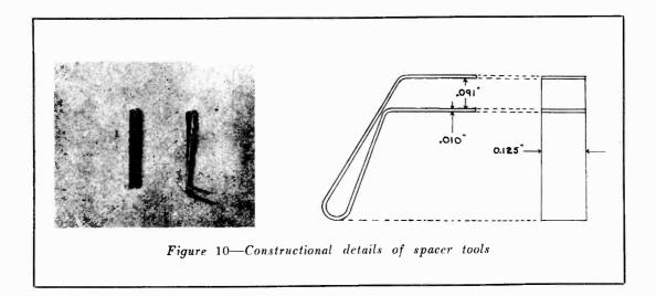
armature correctly it will be first necessary to make a set of spacer tools (Figure 10). These are made of  $\frac{1}{8}$ " stock phosphor bronze .010" thick and bent to give two surfaces .091" apart. Two of these tools are necessary. After the two screws are loosened at each end of the armature these tools are inserted at each end between the armature and pole pieces (Figure 11). The screws are then tightened with the spacer tools in place. This completes the adjustment.
