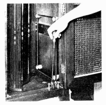
Figure 7-Connecting antenna and ground leads to the antenna coupler terminals
