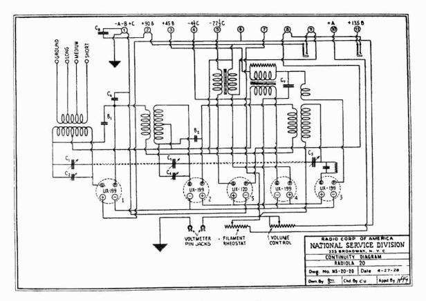
Figure 4-Continuity wiring diagram
