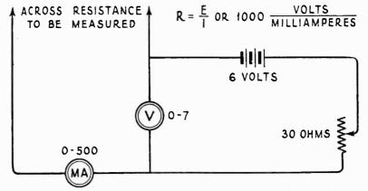
Figure 10-Schematic circuit diagram for resistance measurement
