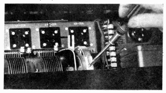
Figure 24—Method used in replacing dial scales.
