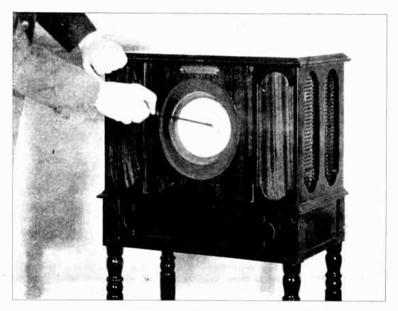
Figure 4-Readjusting cone
