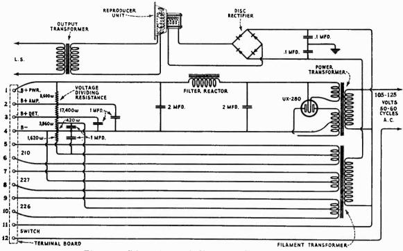
Figure 7—Schematic circuit diagram of Sterling S. P. U.
