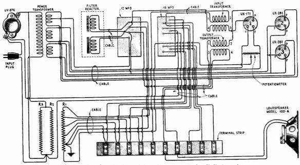
Figure 19-Continuity wiring diagram of the R.P.A. unit
