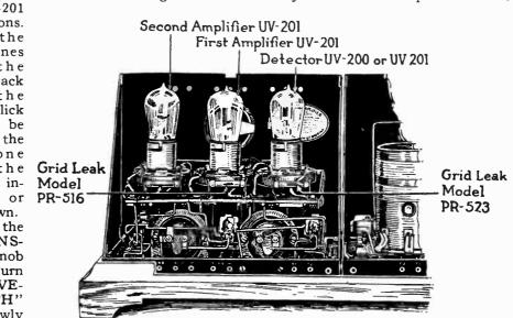
until a signal is heard, and leave it at the point where the signal is loudest. If no signals are heard, or if they are very weak, slowly turn the "INTENSITY" knob clockwise, still searching for signals with the "WAVELENGTH" knob.
