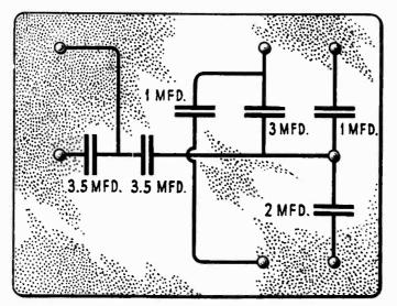
Figure 17—Internal connections of filter condensers.
