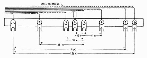
Figure 2-Radiola 25 Battery Terminal Strip
