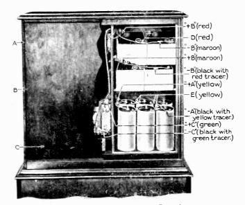
Fig. 1. Rear View, Showing Battery Connections
