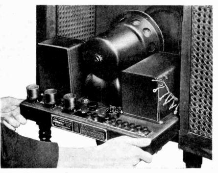
Figure 10-Removing chassis assembly from cabinet.
