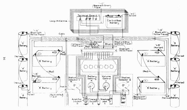
Fig. 6. Connection Diagram of Radiola Super-Heterodyne
