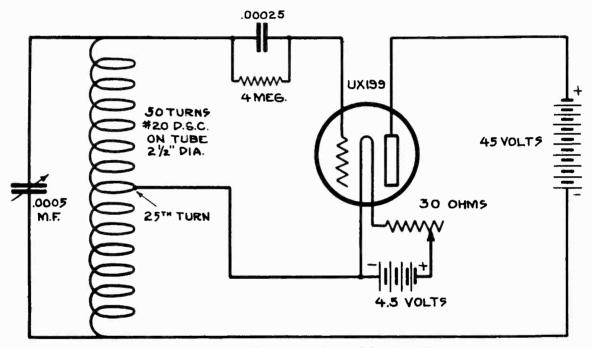
Figure 4-Wiring diagram of the modulated oscillator
