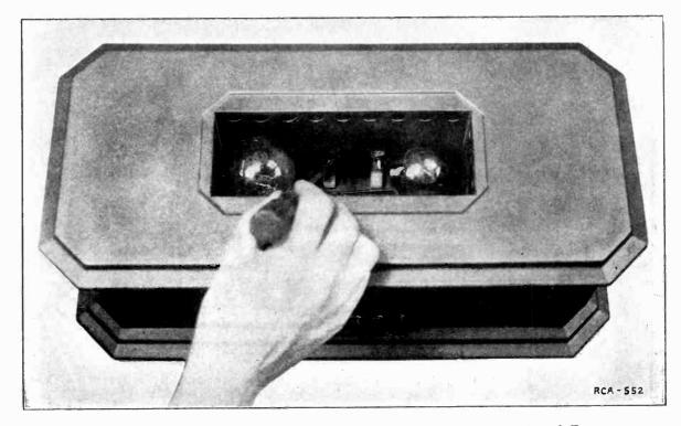
Figure 1-Screw driver used to test magnetic pull of chokes A and B.
