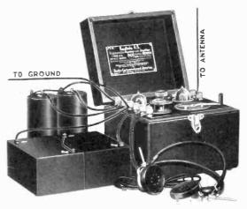
Fig. 2-Radiola RS Connected
