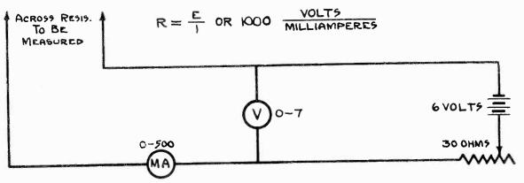
Figure 2-Wiring diagram for resistance measurement
