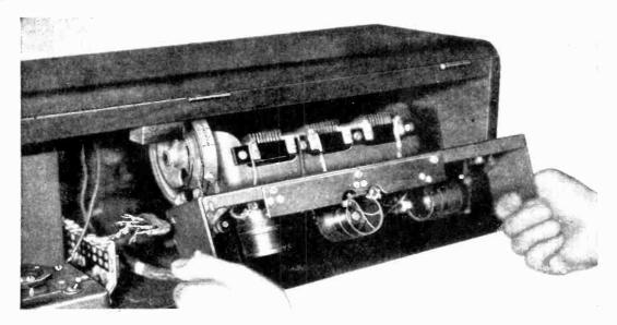
Figure 12—Removing receiver chassis assembly from cabinet.
