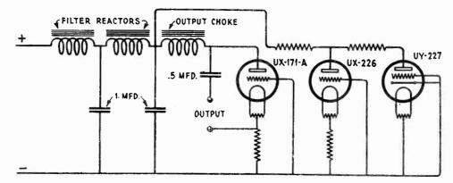
Figure 9—Schematic circuit illustrating method of obtaining grid and plate voltages.
