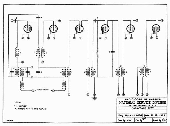
Figure 1 Continuity test circuit of standard six-tube catacomb
