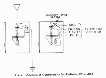
condenser of the RADIOLA RT to tune the loop circuit. It is practically necessary to use radio frequency amplification with a loop. In connection with the portable loop model HG 1380 a wavelength range sufficient to take in the broadcasting stations will be obtained. Fig. 6 shows the connections.
