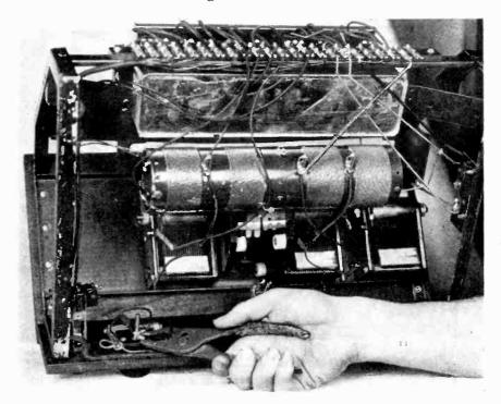
Figure 4-Adjusting contact arm on rheostat
