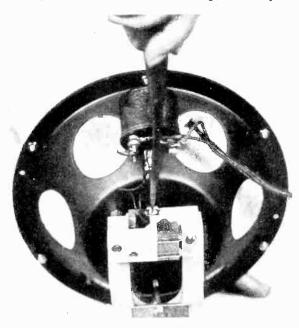
Figure 15-Adjusting the thrust lever screw
