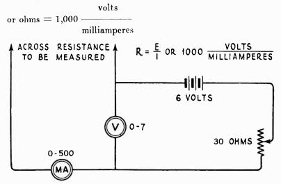
Figure 9-Schematic circuit diagram for resistance measurement
