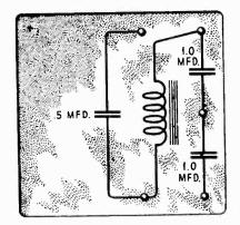
Figure 8—Internal connections of condensers.
