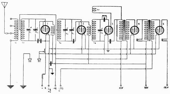
Figure 1—Schematic circuit of RCA Radiola 20
