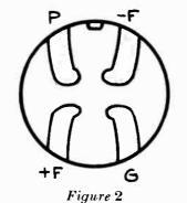
Radiotron UV-199 Socket Terminals
