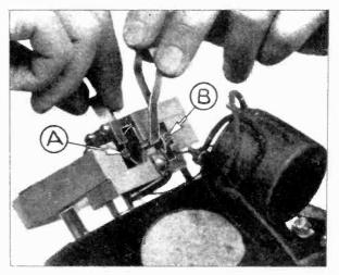
Figure 13—Armature bracket adjusting screws A and B
