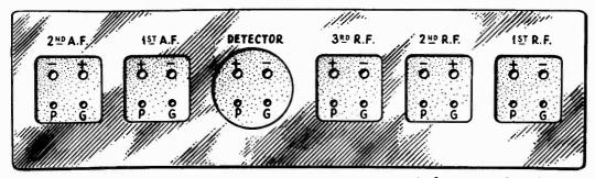
Figure 7—The correct filament polarity of the various Radiotron sockets in RCA Radiola 16
