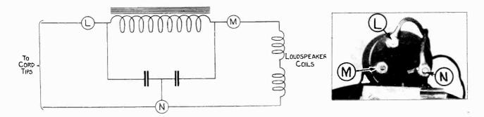
Figure 8-Schematic circuit diagram of RCA Loudspeaker Model 100.4 and photo of the filter unit
