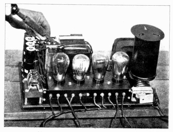
Figure 5-Testing 2 Mfd. condensers for leakage
