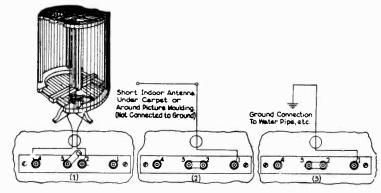
Fig. 5. Connection of Exterior Loop, Indoor Antenna, etc.
