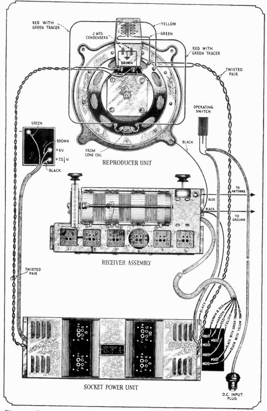
Figure 6—Complete layout and connections of reproducer, receiver and socket power unit 10
