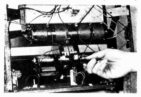
Figure 5-Adjusting friction shaft clutch tension screw inside of tuning drum assembly
