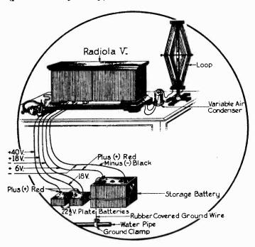
to the negative (-) of the 40-volt plate battery, omitting the connections from the "-40 V." terminal of the receiver to the plate battery.
