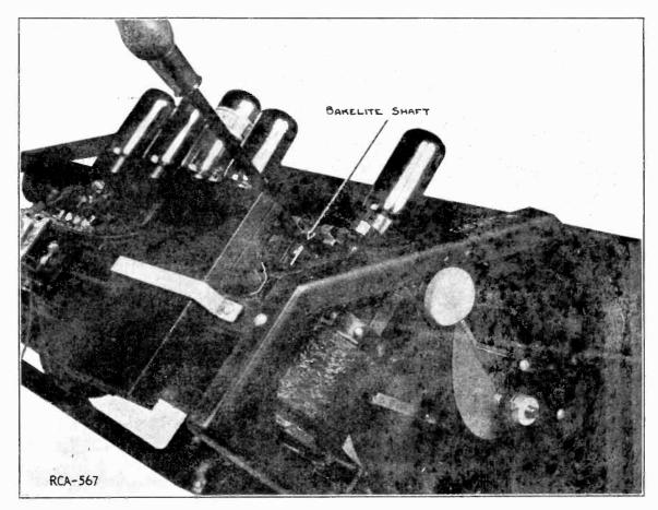
Figure 5 Illustrating method of adjusting first neutralizing condenser
