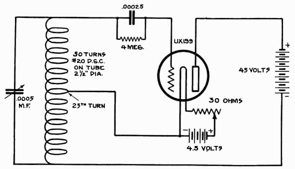
Figure 4-Wiring diagram of the modulated oscillator
