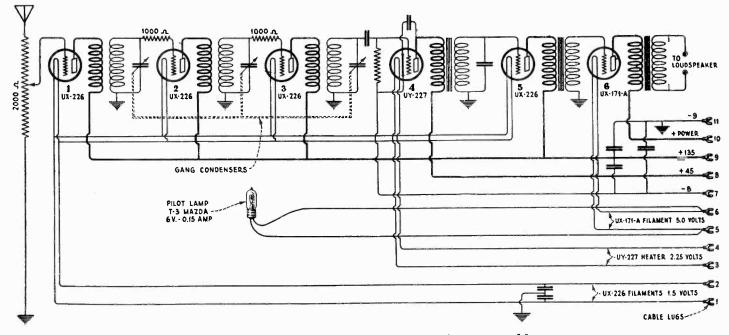
Figure 4-Schematic circuit diagram of receiver assembly.
