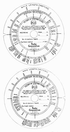
Fig. 4. "STATION SELECTOR" Dials, Showing Approximate Markings of Principal Broadcasting Stations
