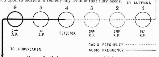
Figure 3-Radiotron sequence in RCA Radiola 17
