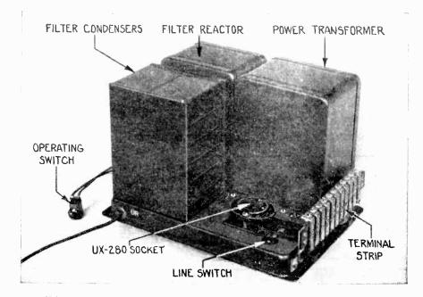
Figure 2-Socket Power Unit showing various parts.
