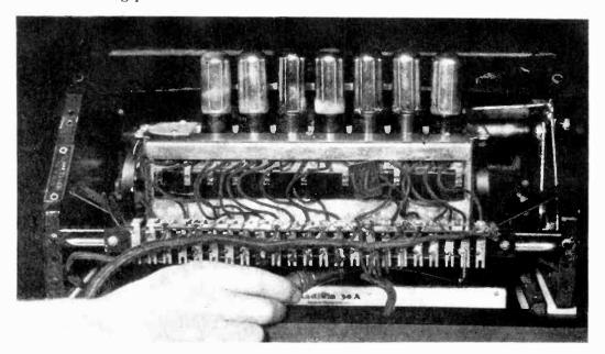
Figure 7-Adjusting neutralizing condenser
