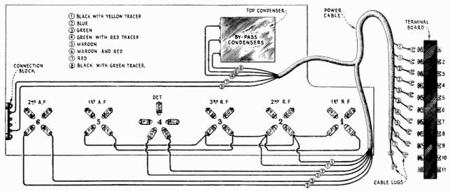
Figure 25—Color scheme of power cable connections.
