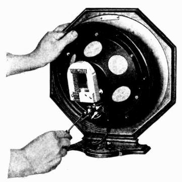
Figure 11—Removing reproducer assembly from baffle
