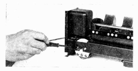
Figure 7-Releasing mounting screws holding volume control.
