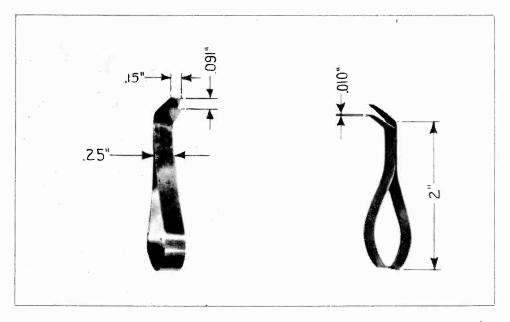
Figure 4—General appearance and correct dimensions of armature spacing tools
