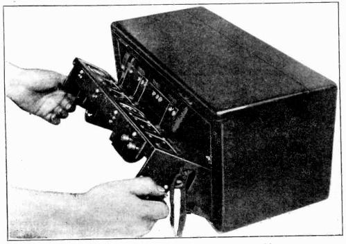
Figure 8-Removing chassis assembly from cabinet
