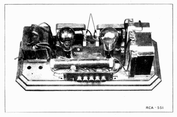
Figure 2-Top view of "B" Battery Eliminator with cover removed and showing arrows where magnetic pull of chokes may be tested.
