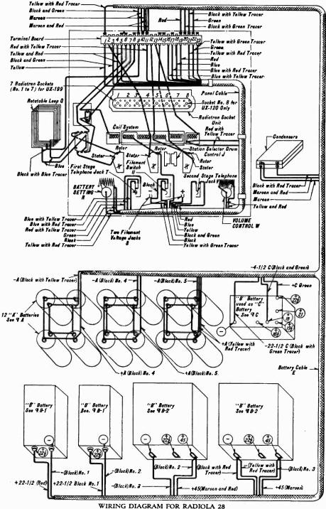
In this wiring diagram, two or more leads of a like color contained in the same cable may be distinguished by the numeral following the color designation at each end of a given lead.
