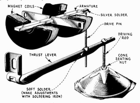
principle of the reproducer unit Figure 14—Diagram showing constructional details and operating
