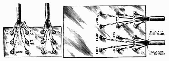
Figure 12—Receptor S. P. U. terminal board and color of connections
