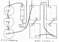
Diagram of Battery Connections for Portable Unit
