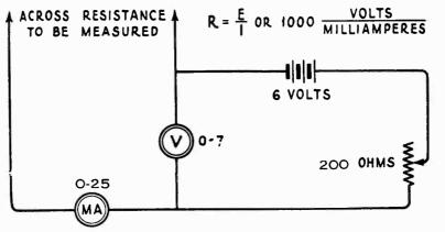
Figure 6-Schematic circuit for resistance measurement
