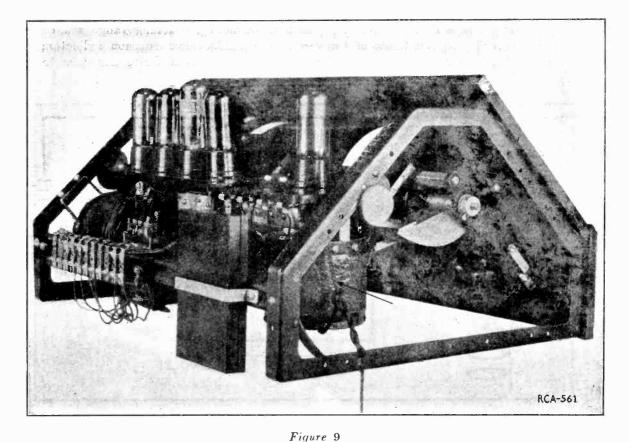
Location of "pick-up" wire for last step in lining up main tuning condensers Radiotrons shown in their correct position
