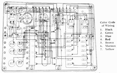
Bottom of Power-Amplifier Unit, showing wiring between terminals
