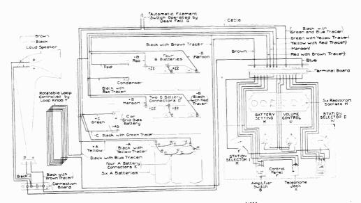
Fig. 5. Connection Diagram of Radiola Super-VIII
