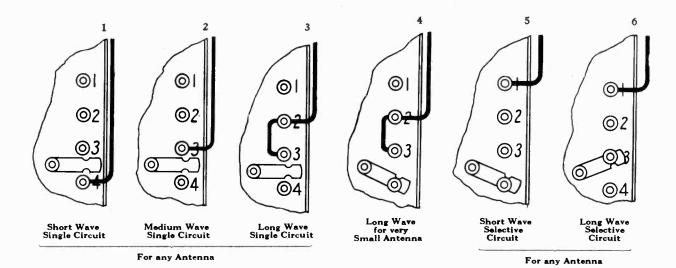
Fig. 3—Showing Antenna Connections to Different Binding Posts
