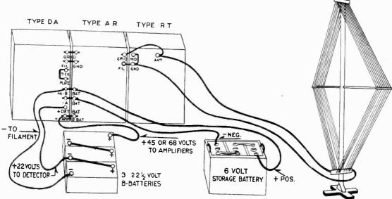
Fig. 6—Radiolas RT, AR and DA with Loop
