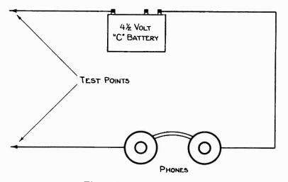
Figure 3—Click test circuit
