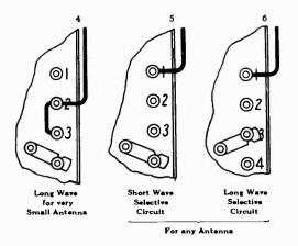
Fig. 3-Showing Antenna Connections to Different Binding Posts
