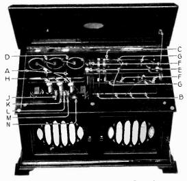
Fig. 1 Interior View Showing Battery Connections
