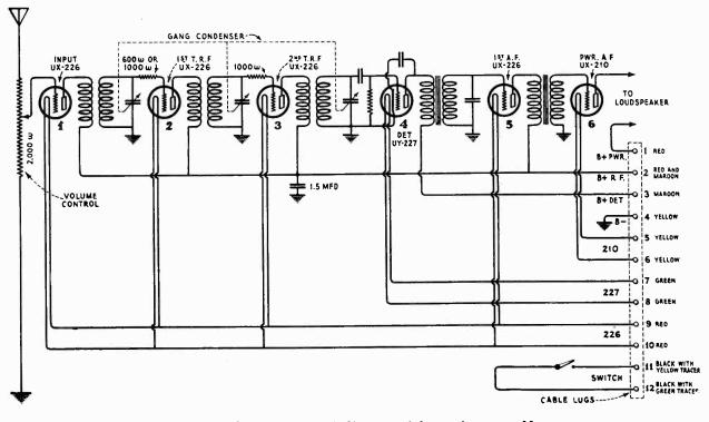
Figure 6—Schematic circuit diagram of the receiver assembly in Radiola 41
