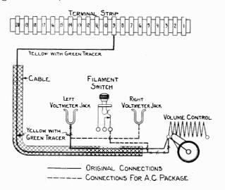
Figure 3—Pancl wiring change required for installation of UP-971 in some models of Radiola 25
