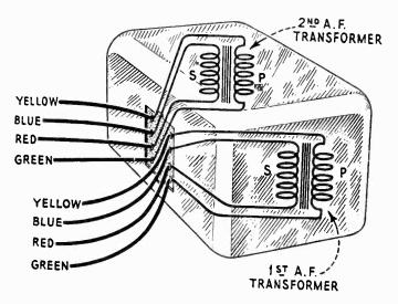
Figure 14-Internal connections of A. F. transformers
