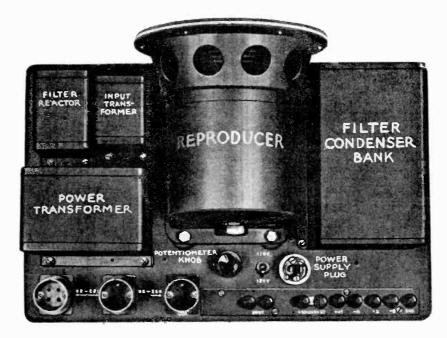
Figure 2—Top view of chassis assembly.
