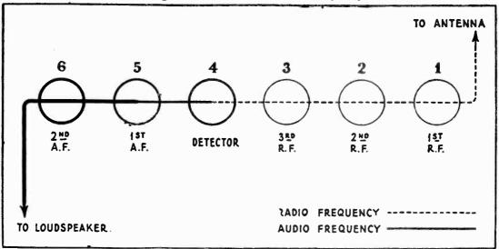
Figure 2-Radiotron sequence in RCA Radiola 16
