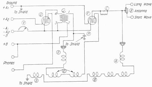
Fig. 6—Diagram of Connections Radiola RS
