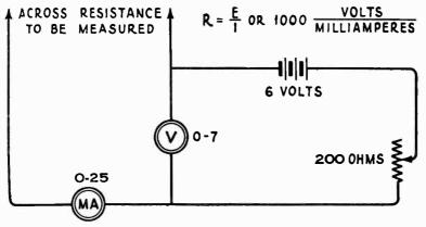
Figure 12—Schematic circuit for resistance measurement. The resistance may then be calculated by the use of Ohms law.  $\mathbf{R} = \frac{\mathbf{E}}{\mathbf{I}} \begin{pmatrix} \text{Where R equals ohms} \\ \mathbf{E} \text{ equals volts and I equals amperes} \end{pmatrix}$  or 1000  $\frac{\text{Volts}}{\text{Milliamperes}}$
