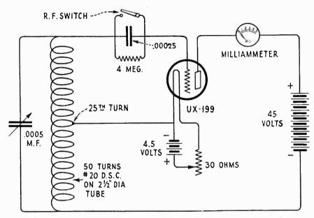
Figure 4—Schematic circuit diagram of the radio frequency and audio frequency oscillator
