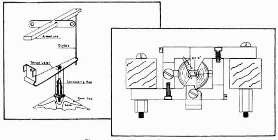
Figure 9-Details of loudspeaker unit
