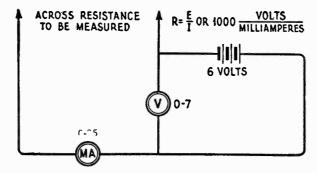
Figure 9—Schematic diagram of resistance measurement method
