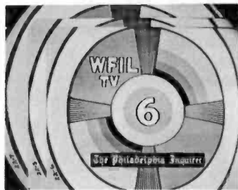
Fig. 2. Effect of line voltage on picture width and height is shown by these three superimposed photographs taken with line voltages of 105, 115, and 125 volts. The picture size is smallest with 105 volts, and largest with 125 volts. When sufficient width cannot be obtained by means of the width and drive adjustments, it is advisable to check the line voltage.
