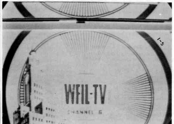
Fig. 5—Low-frequency phase shift. 1st-video grid resistor dropped from 470,000 to 3000 ohms. The contrast was turned down, brightness turned up, and vertical hold control adjusted to show vertical blanking and sync. Note trailing reversal after vertical sync, and after vertical blanking.
