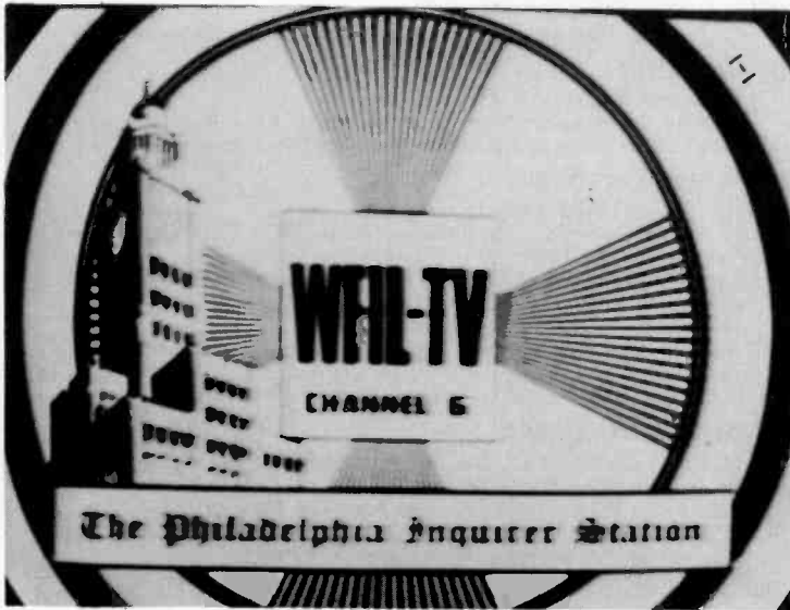
Fig. 2—This shows normal conditions. There is a slight trailing light-grey smear on the right-hand side of the lettering, and after the lines in horizontal wedge.
