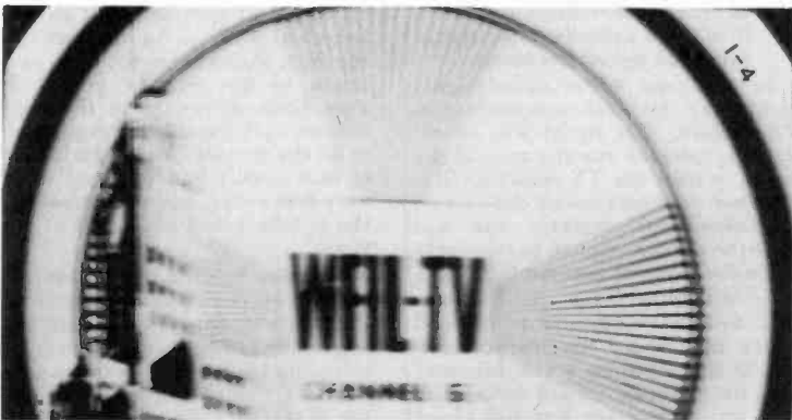
Fig. 8—Excessive low-frequency response. 1st- or 2nd-video plate load of 3300 ohms increased to 10,000 ohms. Increases low-frequency response, decreases highs. General smearing of both wedges except center lines in horizontal wedge. Same general effect as shown in Figs. 4 and 6.
