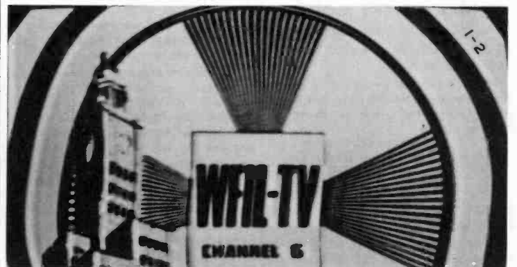
Fig. 9—Trailing reversal, white after black, produced by 2nd-video cathode resistor increasing from 330 ohms to 1500 ohms. Resulting incorrect bias makes it difficult to obtain suitable contrast.
