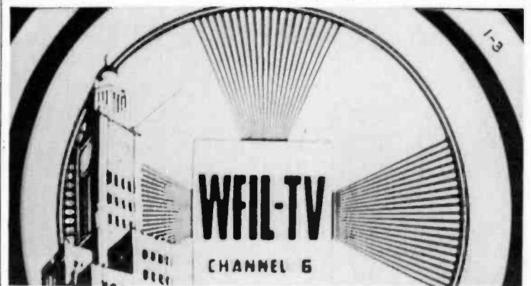
Fig. 7—Excessive high-frequency response. 1st- or 2nd-video plate load of 3300 ohms dropped to 1000 ohms. Reduces low-frequency response, exaggerating highs. Note trailing reversal, white followed by a fine dark line, after lettering.
