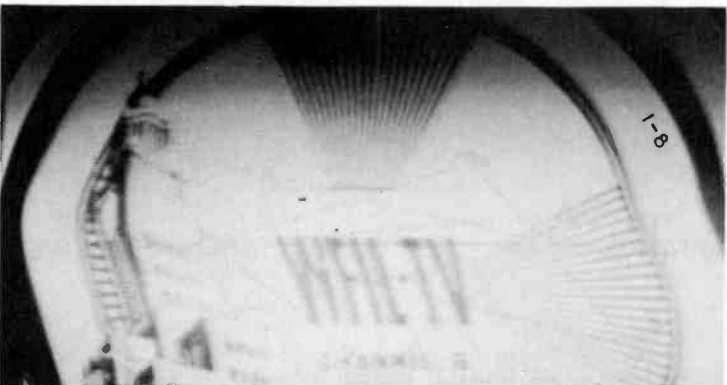
Fig. 10—Hum in video, produced by heater-cathode leakage (700 ohms) in 2nd video stage. Hum voltage darkens some portions and lightens other portions of picture. Hum also gets into horizontal-sync, distorting shape of picture.
