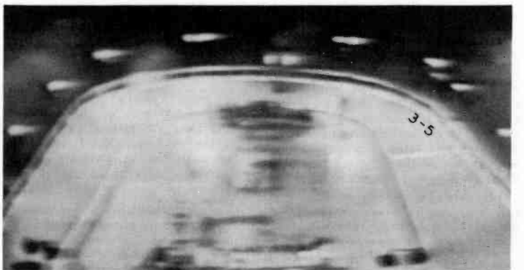
Fig. 13—Believe it or not, this is a roller-skating rink. The smearing is not caused by trouble in the receiver, but by unusually poor TV relay conditions. Moral. Don't tear the set apart until reception has been checked on other stations or on other receivers.
