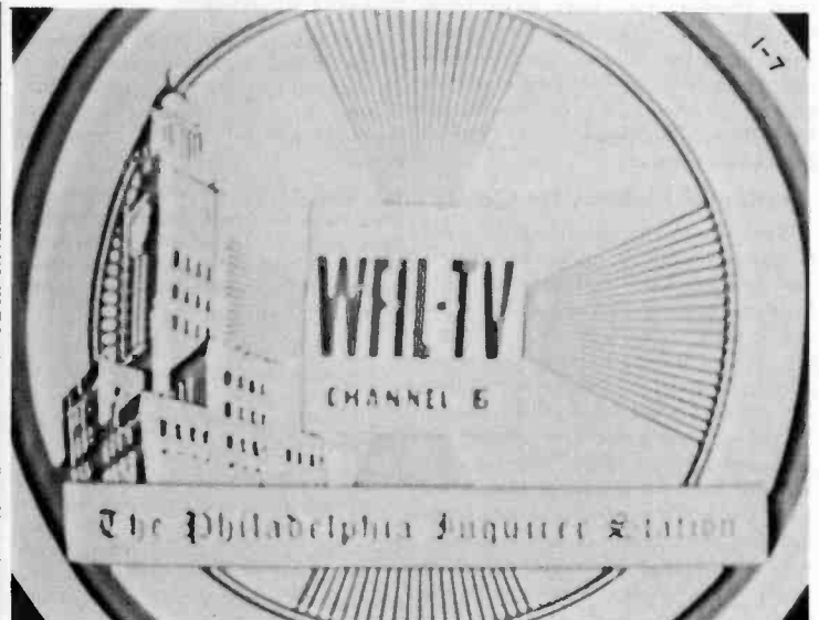
Fig. 3—Poor low-frequency response. 2nd-detector load resistor, not shown in schematic, dropped from 3900 to 100 ohms. Note trailing reversal, white after black, on right-hand side of lettering. Lettering and outer circle are not uniform.
