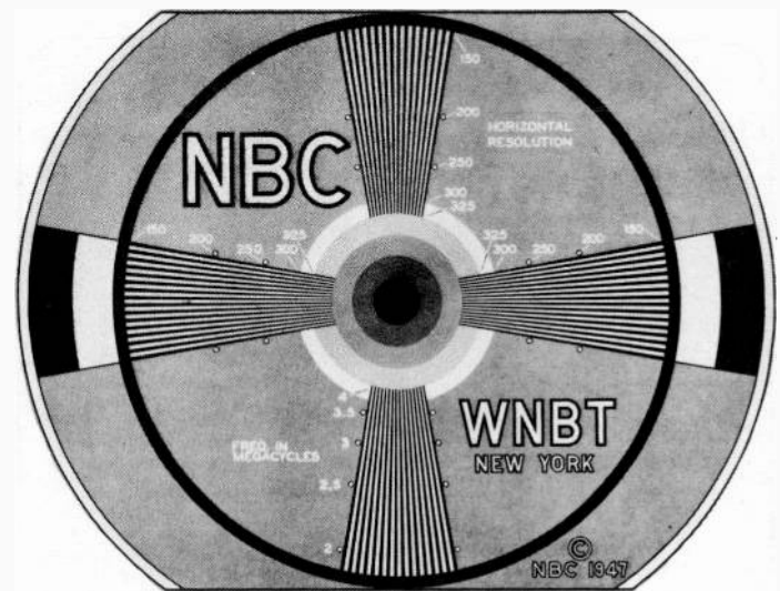
Figure 8. The NBC Test Pattern, showing the equivalent frequency and number of lines at the major points on the wedges.
