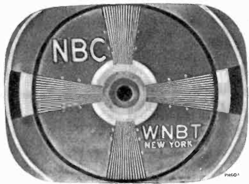
Figure 21—Focus Magnet and Ion Trap Magnet Misadjusted
