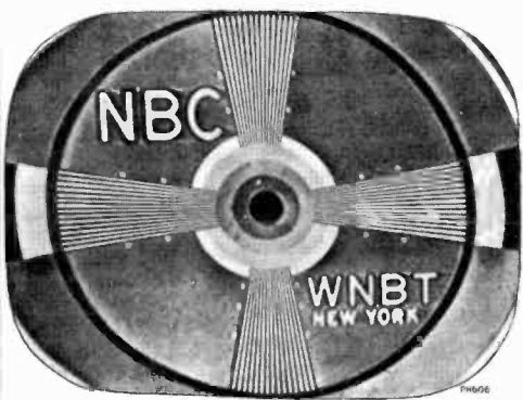
Figure 22—Horizontal Linearity Control Misadjusted (Picture Cramped in Middle)
