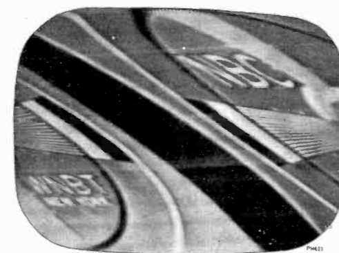
Figure 26—Test Pattern Showing Out of Sync Condition When Horizontal Hold Control Is in a Counter-clockwise Position—Just Before Pulling Into Sync
