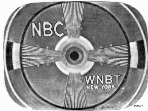
Figure 21—Focus Magnet and Ion Trap Magnet Misadjusted
