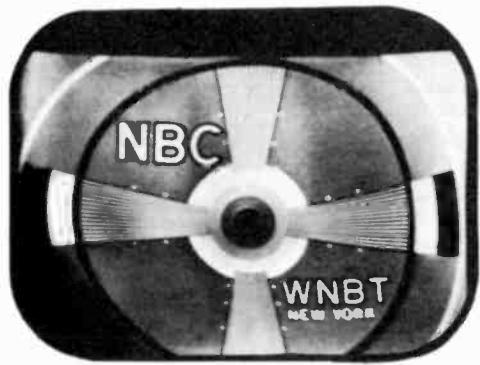
Figure 22—Focus Coil and Ion Trap Magnet Misadjusted
