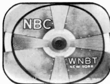
Figure 24—Horizontal Linearity Control Misadjusted (Picture Cramped in Middle)
