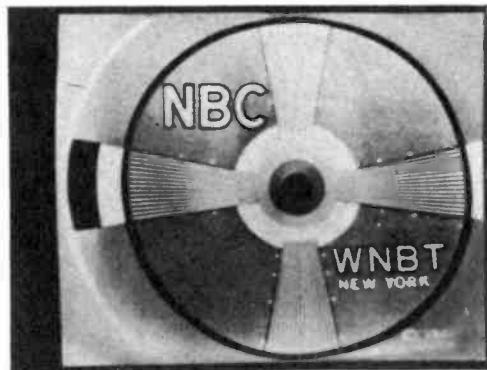
Figure 52—Electrical Horizontal Centering Control Misadjusted
