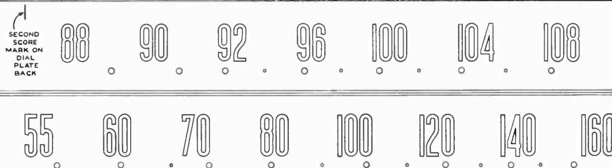
The dial scale drawing shown is a full size reproduction. It can be used as a reference during alignment.
