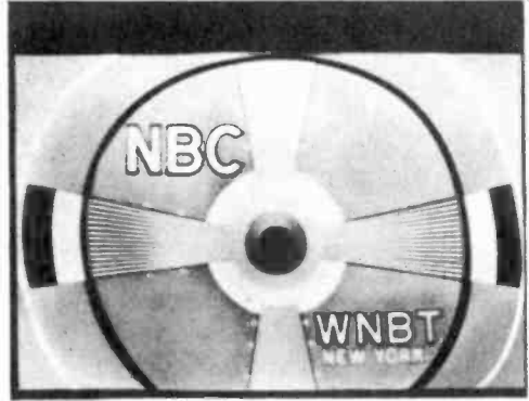
Figure 52—Electrical Horizontal Centering Control Misadjusted
