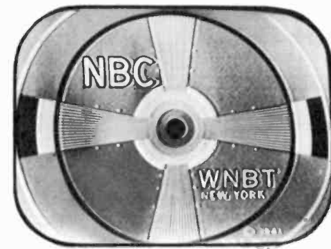
Figure 25—Horizontal Drive Control Misadjusted
