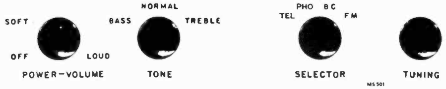
Figure 11—Radio Panel Controls
