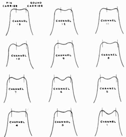
Figure 17—Typical R-F Response Curves
