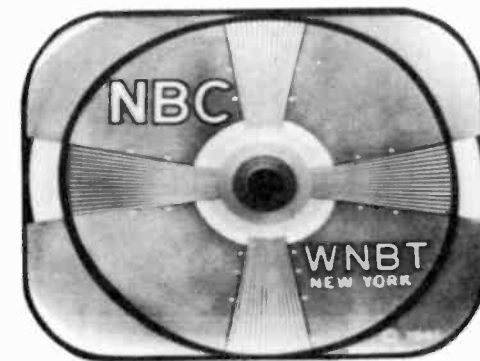
Figure 23—Horizontal Linearity Control Misadjusted (Picture Cramped in Middle)
