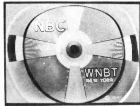
Figure 54—Vertical Linearity Control Misadjusted
