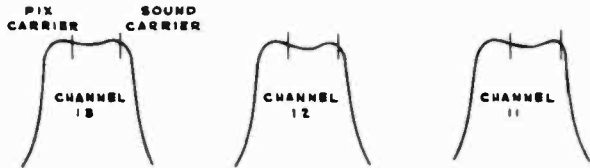
Figure 30—Sound Discriminator and I-F Response
