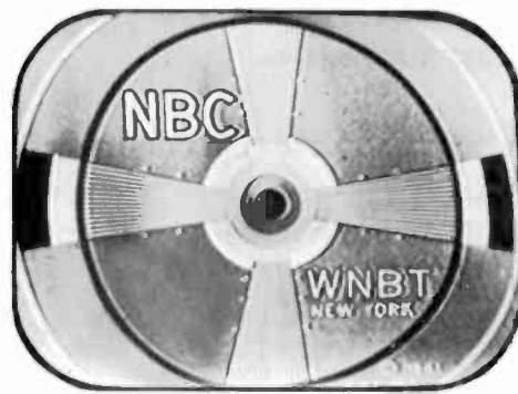
Figure 26—Horizontal Drive Control Misadjusted
