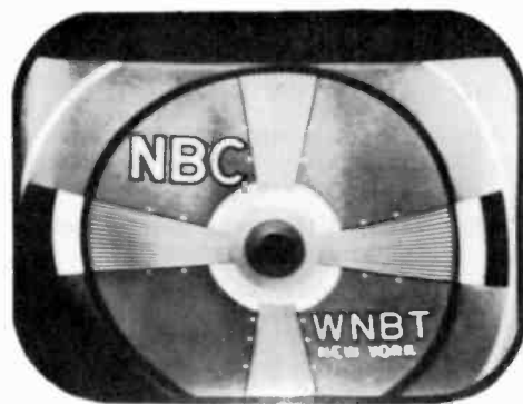
Figure 23—Focus Coil and Ion Trap Magnet Misadjusted
