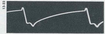
8B. Normal waveform, without a TV signal. A CRO sweep rate of 5,250 cycles was used for all photographs in this column.
