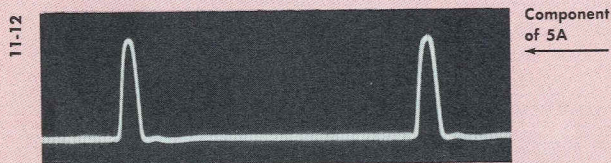
5C. This component of 5A is the "stray" horizontal flyback pulse, shown in 4H, after it is amplified and inverted in the 2nd-sync separator. (C1 was opened, for this photograph, in order to eliminate the component shown in 5B.)
