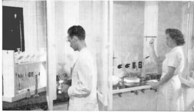
R. H. Plumlee, physical chemist, and Mrs. W. F. Kaser, laboratory assistant, analyze and mix purified phosphor constituents. Compartments prevent cross-contamination.
