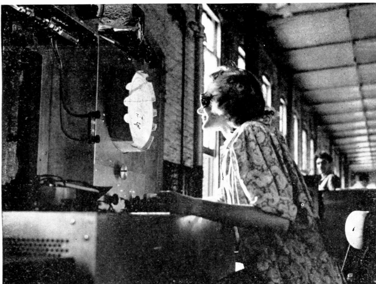
Checking RCA Television Kinescopes for screen characteristics. These characteristics include brilliancy, color, focusing, overall detail, and size of the picture. Every Kinescope receives this individual test. The equipment used for checking these characteristics is capable of producing up to 12,000 volts for the handling of all sizes of Kinescopes.
