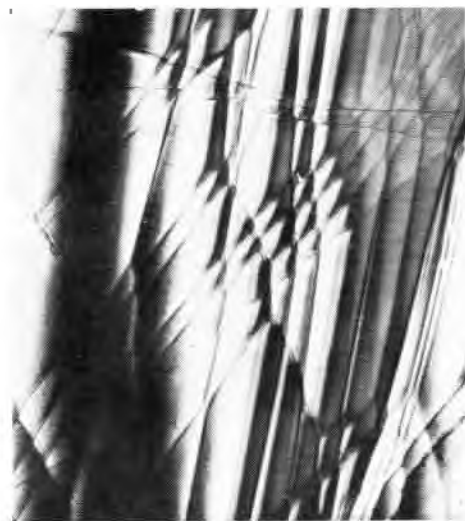
TYPICAL MICROGRAPH taken on the RCA EMU-3; Bismuth Telluride magnified 9,000X
